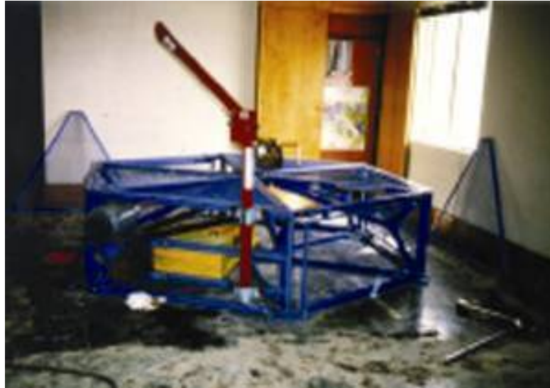
Figure 5: Forced vibration oscillator setup
