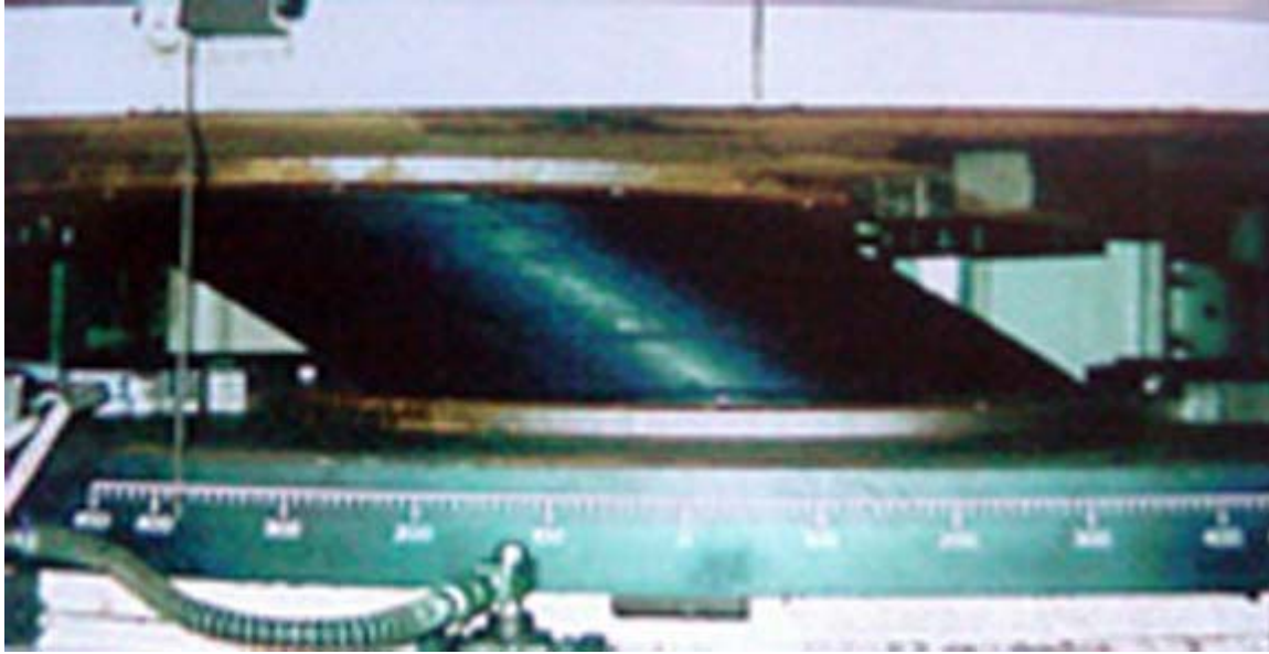
Figure 9: Shear displacement test of bearing
