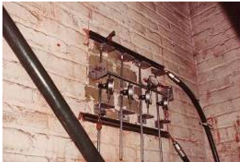
Figure 6: URM in-stu test setup
