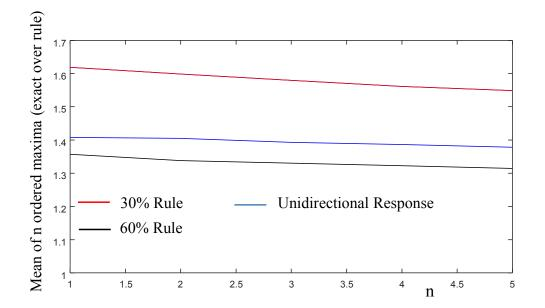
Fig.13. Mean of ordered maxima of the ratio of exact to estimated response based on 100 simulations for building of Fig.12with 2% damping.
