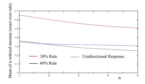
Fig.14. Mean of ordered maxima of the ratio of exact to estimated response based on 100 simulations for building of Fig.12 with 5% damping.
