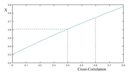
Fig.11. Value of X in the 100+X% rule for which the maximum response is "correctly" estimated vs the cross correlation between bi-direction responses.
