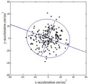
Fig.1. Accelerations, principal directions and inscribing ellipse for the first 4 sec window in the strong motion defined using the to.9 Arias Intensity.
