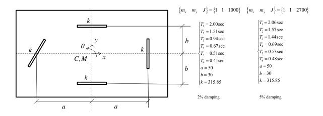
Fig.12. Plan view and periods of the 10 story shear buildings used in the validation study, damping is 2% in all the modes.
