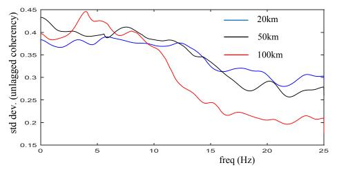
Fig.5. Standard deviation of the unlagged coherency vs frequency, M = 7.5, Strike-Slip,  $V_{s30}=500$  m/sec.
