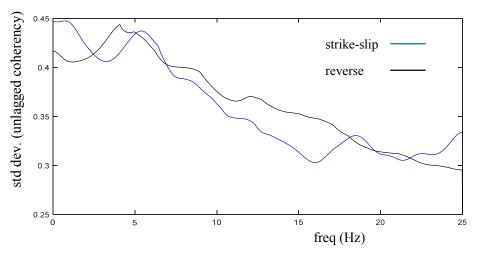
Fig.4. Standard deviation of the unlagged coherency vs frequency, M = 7.5, R = 40Km,  $V_{s30}$ =500 m/sec.
