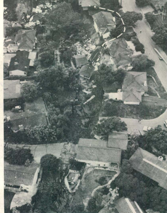
Photo 3. Aerial photo of headscarp area taken the day of the slide (October 2, 1978). Dashed outline is the area which failed 10 days later, illustrating the instability of the ground behind the October 2 headscarp. View looking northeast. Courtesy of City of Laguna Beach.
