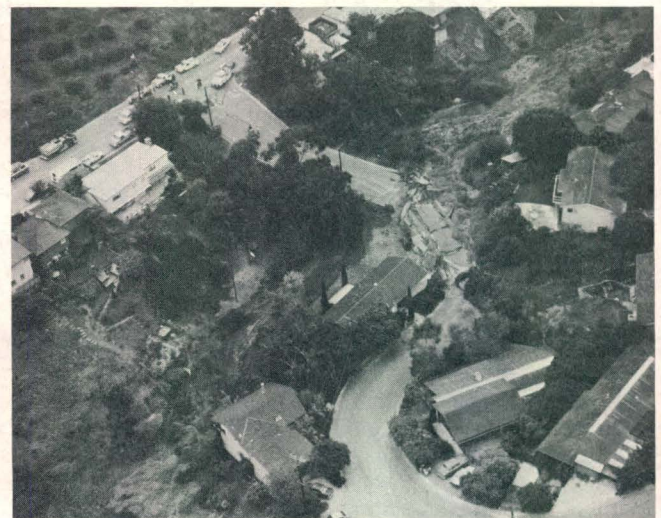
Photo 5. Aerial photo of easternmost toe area of slide. Note butting effect of road fill ("af" on figure 1) where Oriole Drive crosses Bluebird Canyon. View toward the southwest. Photo courtesy City of Laguna Beach.
