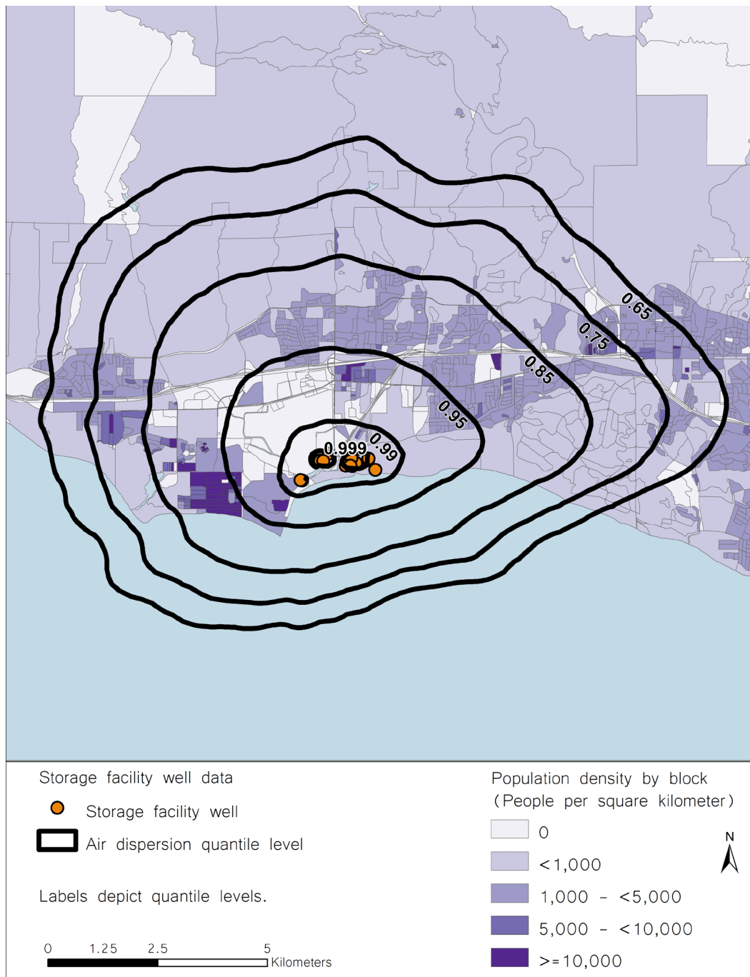
Figure 1.4-14. Air dispersion quantiles and population density at the La Goleta UGS facility.
