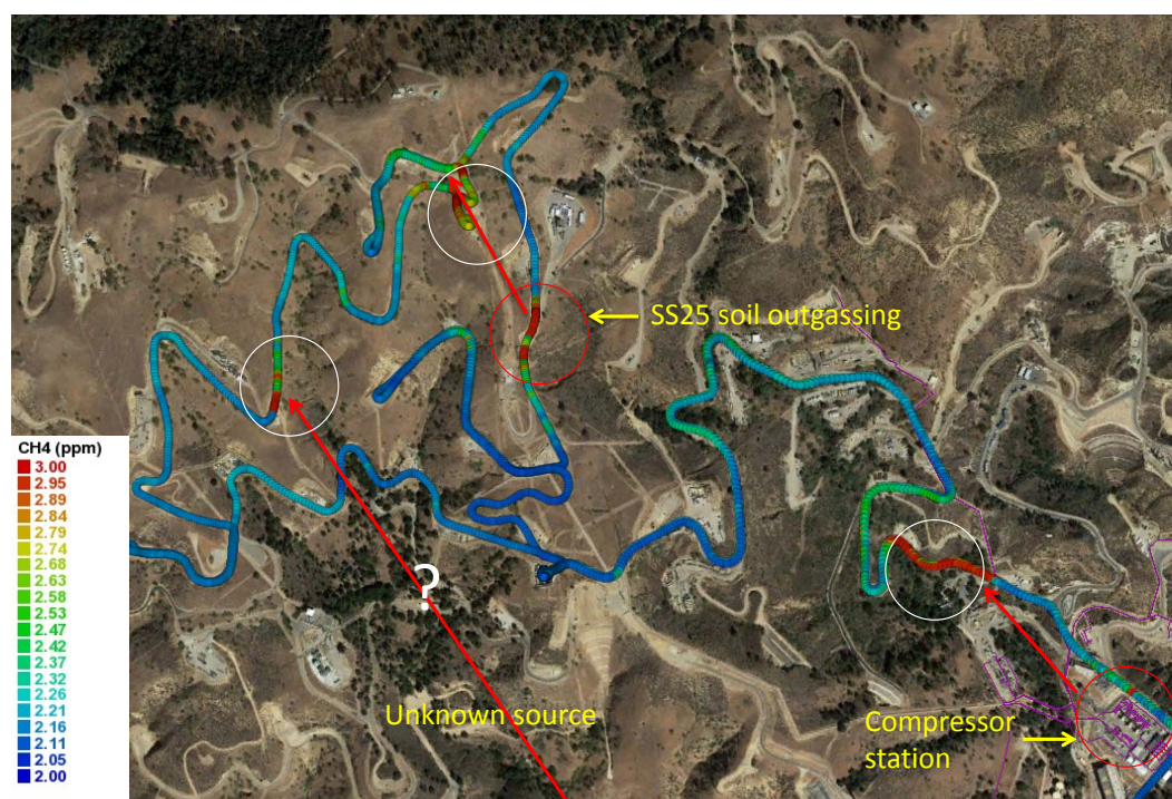
Figure 1.5-7. Example of an on-road methane survey using an in situ methane analyzer. The color scale indicates near-surface methane mixing ratios. Data were collected on July 8, 2016, roughly five months after the SS-25 leak was plugged. The facility was in a shut-in state. The red arrows indicate prevailing wind direction. This reveals several methane hotspots that exceed normal background levels, consistent with gas plumes crossing the roads. There were two likely methane sources: residual soil outgassing from the SS-25 incident and the facility's compressor station. The former is expected given earlier measurements of soil methane levels there. The latter suggests either venting associated with maintenance or a leaking component at the compressor station. The source of the third methane hotspot observed to the west is unclear. There are multiple UGS and producing and abandoned oil wells along the red arrow that could be responsible (data courtesy SCAQMD).
