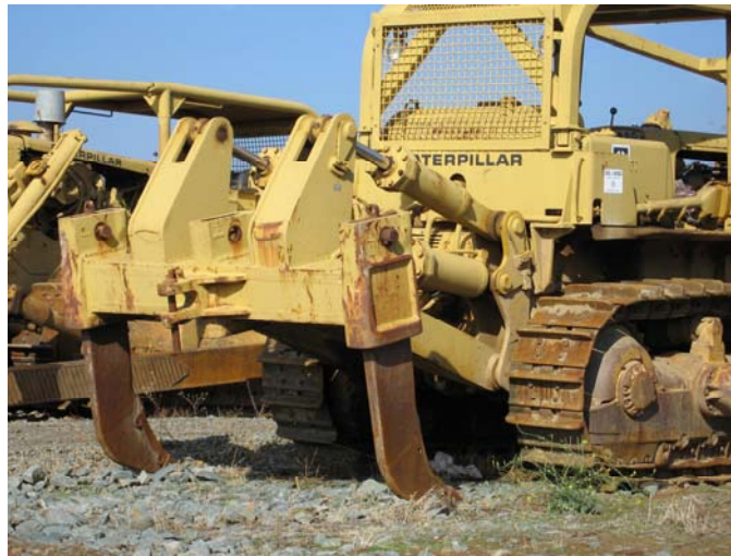
Caterpillar tractor with ripping shanks.
