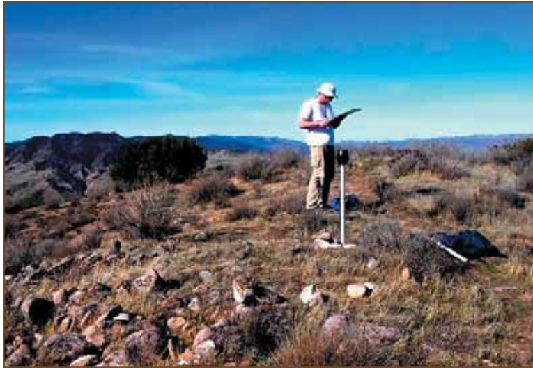
Taking notes at a new automatic recording rain gauge in Griswold Hills.
