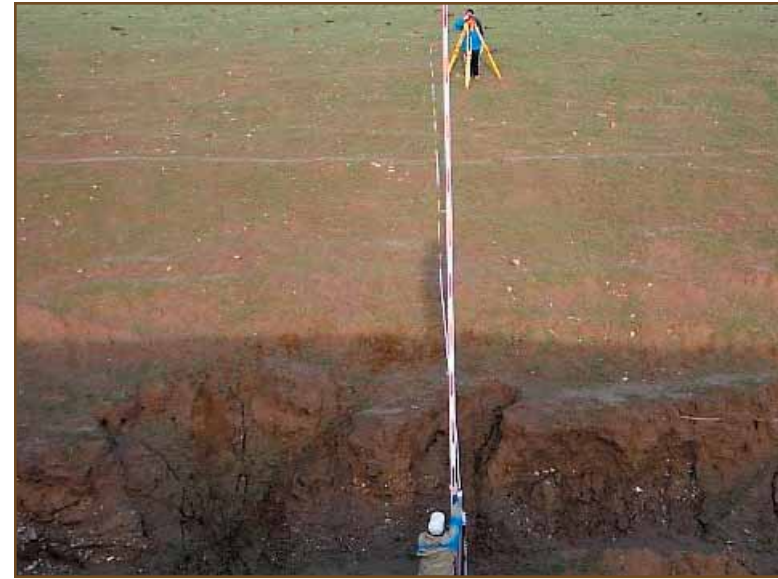
Surveying a channel cross section for crest stage gauge setup on Panoche Creek.
