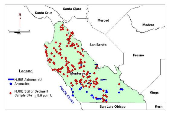
Figure 6. Comparison of NURE Airborne Survey eU Anomaly Locations with NURE Soil and Sediment Sample U Anomaly Locations
