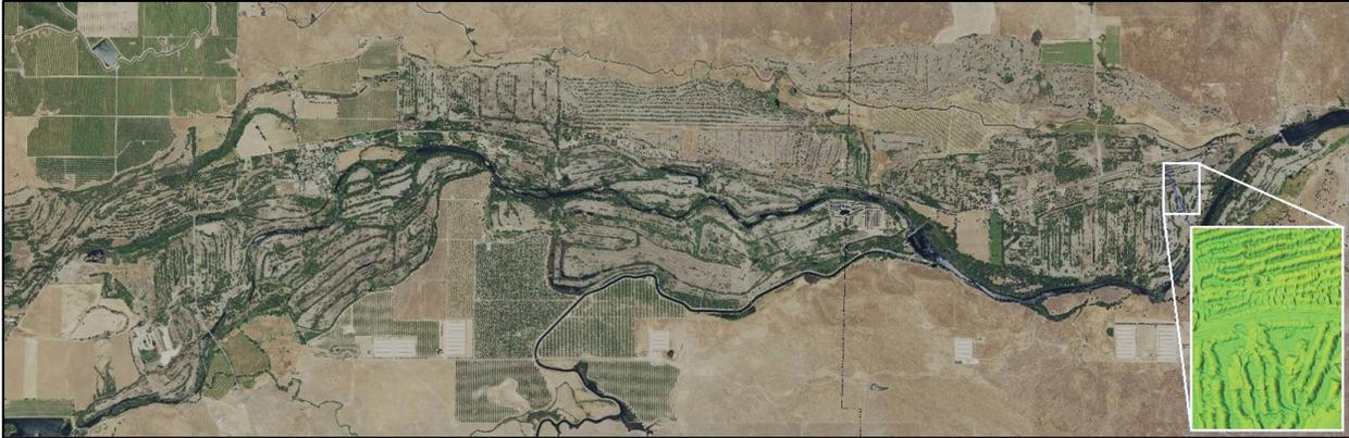
**Figure 5.** Aerial photo of a portion of the Snelling dredge field, on the Merced River. Arcuate pattern of tailing windrows (visible in photo inset) is produced by the dredge stacker oscillating back and forth ejecting coarse sediments (gravel and boulders) as the dredge moves forward. Finer material is ejected back into the dredge pond separately. (Main image from 2020 NAIP; inset from lidar-derived shaded relief image).
