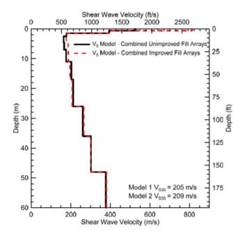
Figure 9a: Comparison of shear wave velocity profiles across the Berth 404 site (GEOVision 2013).
