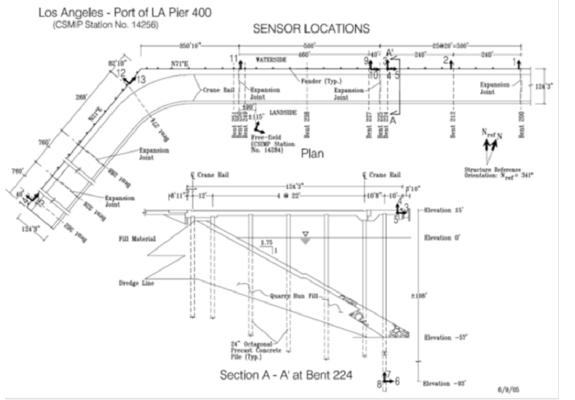
Figure 4: CSMIP Instrumentation Array at the Port of Los Angeles Pier 400 (CGS - CSMIP Station 14256), Center for Engineering Strong Motion Data (CESMD)
