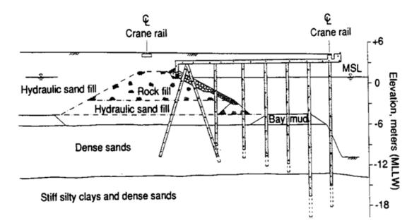
Figure 1. Pile-supported wharf at the Port of Oakland Seventh Street Terminal, prior to the 1989 Loma Prieta Earthquake (Egan et al. 1992).
