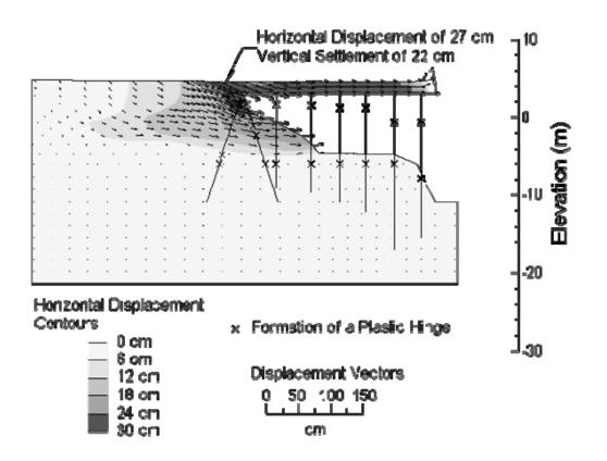
Figure 3. Numerical simulation of seismic performance of Berth 38, Seventh Street Terminal, Port of Oakland during the 1989 Loma Prieta Earthquake.
