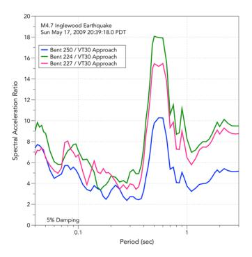
Figure 6b: Spectral amplification ratios for structural response (wharf deck) at Berth 404 and motions recorded at a depth of 100 ft at the Vincent Thomas Bridge West Arrays.
