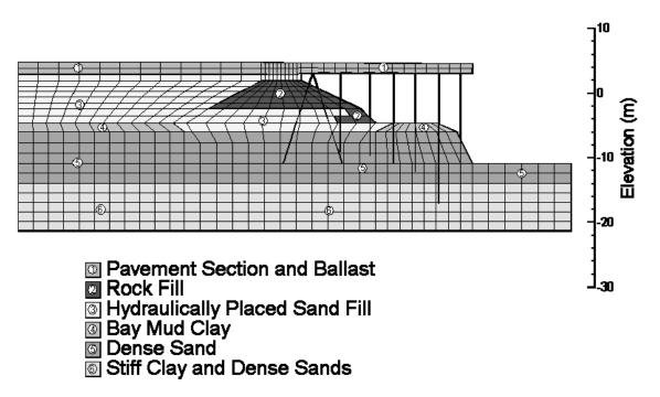
Figure 2. Geometry, grid and structural elements that were used in the numerical model of the Port of Oakland Seventh Street Terminal, Berth 38.
