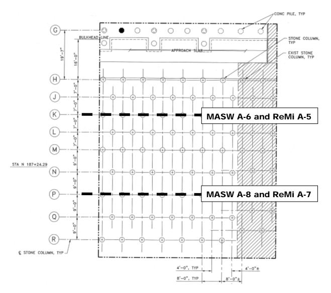
Figure 8: Location of geophysical arrays for surface wave velocity investigation of hydraulic fill treated with stone columns at Berth 404 (after POLA, 2005).
