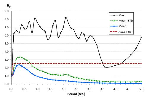
Figure 4. Comparison of Code Values for Component Amplification Factor,  $a_p$ , and Mean, Mean Plus Standard Deviation, and Maximum 5%-Damped  $a_p$  Spectra Calculated Based on 3742 CSMIP Floor Acceleration Histories from Fixed-Base Buildings
