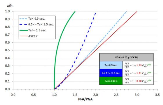
Figure 7. Profile of PFA/PGA over Building Height Recommended for Seismic Design of Acceleration-Sensitive Nonstructural Components in New Constructions under Earthquakes with PGA  $\geq$  0.20 g (SDC D or Higher of Occupancy Category I through III)
