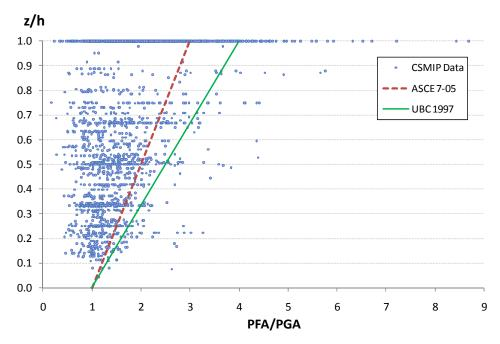
Figure 2. Data Points vs. Building Code Formula for Relationship between PFA/PGA and z/h (2224 above-Ground Level Data Points from 151 Fixed-Base Building Stations)
