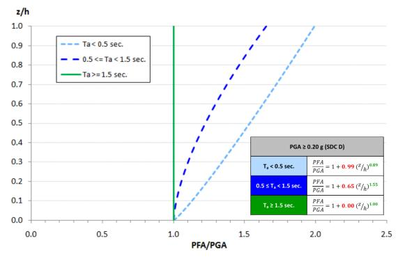
Figure 6. Profile of PFA/PGA over Building Height Recommended for Seismic Evaluation of Acceleration-Sensitive Nonstructural Components in Existing Buildings under Earthquakes with PGA ≥ 0.20 g (SDC D or Higher of Occupancy Category I through III)
