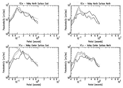
Figure 6. Predicted horizontal pseudovelocity response spectra (dotted lines quartiles) for Valley North (top pair) and Valley Center (bottom pair) surface sites compared with observations (solid lines) (Cramer and Real, 1990b).
