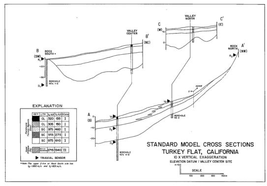
Figure 4. Cross-sections of Turkey Flat Test Area.
