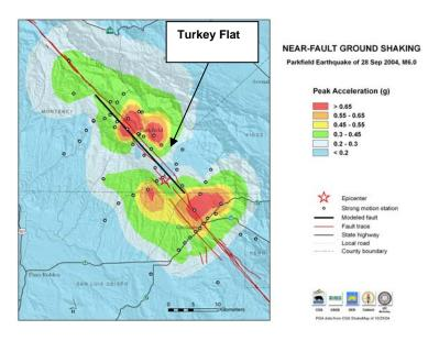
Figure 7. Near-field peak acceleration map of M6.0 2004 Parkfield Earthquake (Shakal et al., 2005)
