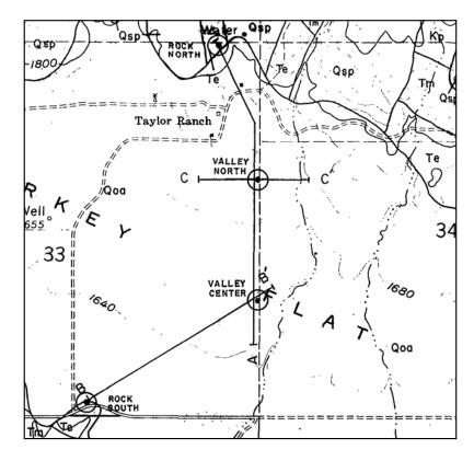
Figure 3. Plan view of Turkey Flat test area showing cross-section lines and location of instrument recording sites.
