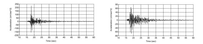
Figure 8. 2004 Parkfield mainshock recorded at (left) Rock South and (right) D3 (rock beneath Valley Center) of the Turkey Flat array.
