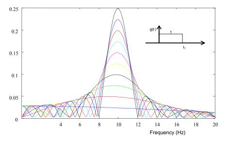
Fig.2 Evolution of the Fourier amplitude spectrum for the signal  $f(t) = sin(20\pi t).g(t,t_1)$  (10 plots corresponding to  $t_1 = 0.05, 0.1, ..., 0.5$  sec).
