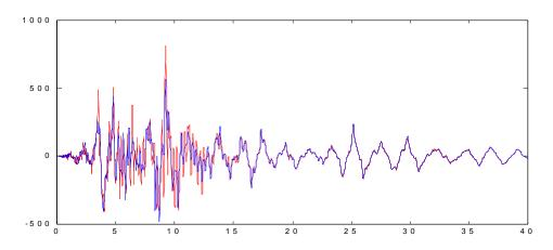
Fig.10. Comparison between measured (blue) and LPO model (red) in channel 9 (cm/sec<sup>2</sup>) Northridge Earthquake
