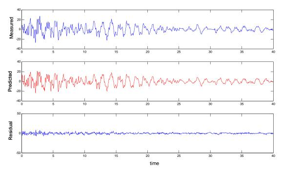
Fig. 7. Comparison of Measured and POM reference accelerations  $(cm/s^2)$  at channel 12 during Big Bear. For illustration, the plot of  $\gamma$  as a function of time for channel 12 is depicted in Fig. 8.
