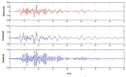
Fig. 9. Measured and PO model reference acceleration (cm/s<sup>2</sup>) in channel 9 during the Northridge Earthquake
