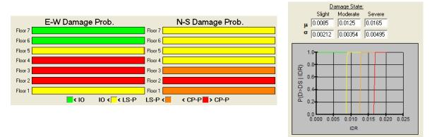
Figure 19. Damage probabilities established using FEMA-356 Tables indicate 100% probability of exceeding Collapse Prevention limit state at second to fourth floors in the E-W direction.
