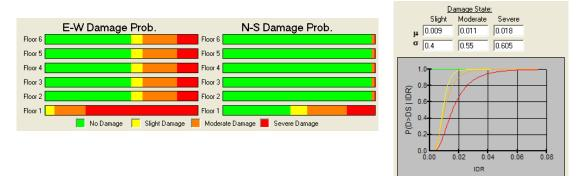
Figure 12. Damage probability established based on PEER/NSF fragility curves for nonductile R/C columns under large gravity loads clearly identifies the first floor columns in the E-W direction as the zone of severe damage.
