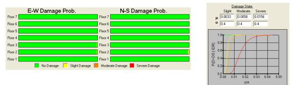
Figure 17. Damage probability established based on HAZUS-MH drift-based fragility curves for older concrete buildings indicates no damage during the Big Bear and Landers earthquakes.
