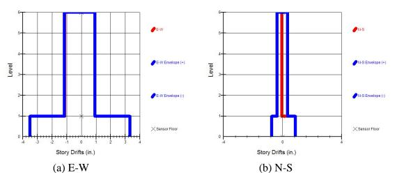
Figure 9. Maximum intersory drifts in the E-W and N-S directions
