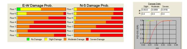
Figure 18. Damage probabilities established based on HAZUS-MH drift-based fragility curves for the 1994 Northridge earthquake show 100% probability of moderate to severe damage at the second to fourth floors.
