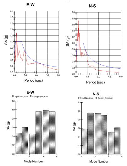
Figure 7. Comparison of the recorded response spectra (5% damped) at the base of the building with a typical "design" spectrum for seismic zone 3 and corresponding elastic modal demands for modes 1 to 3.
