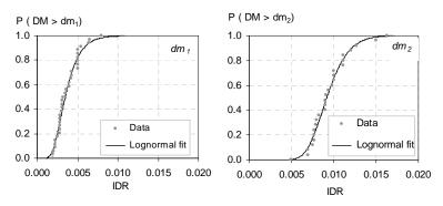
Figure 1. Example of fragility functions to estimate damage in reinforced concrete buildings with slab-column connections as a function of interstory drift (After Aslani and Miranda, 2003).
