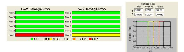
Figure 14. Damage probability established using Tables contained in FEMA-356 for limit-states of nonductile concrete columns clearly identifies the first floor in the E-W direction as the zone of severe damage.
