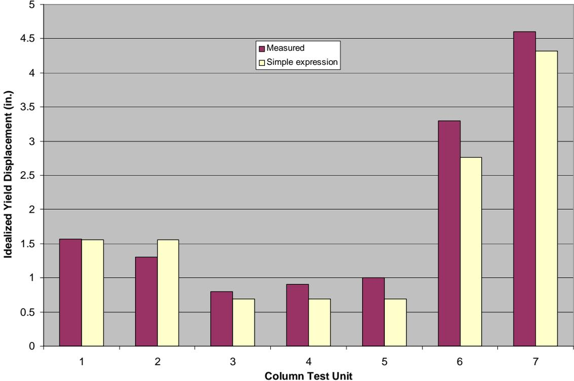
Figure 3. Measured versus simple expression yield displacements
