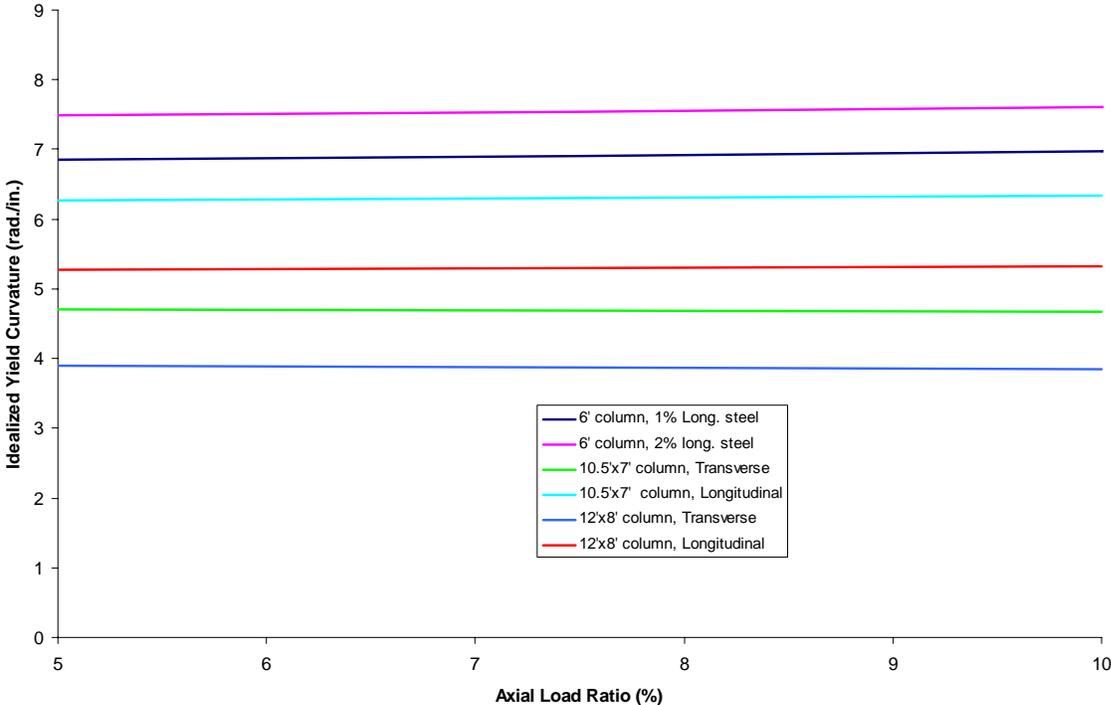
Figure 1. Idealized yield curvature from moment-curvature analyses
