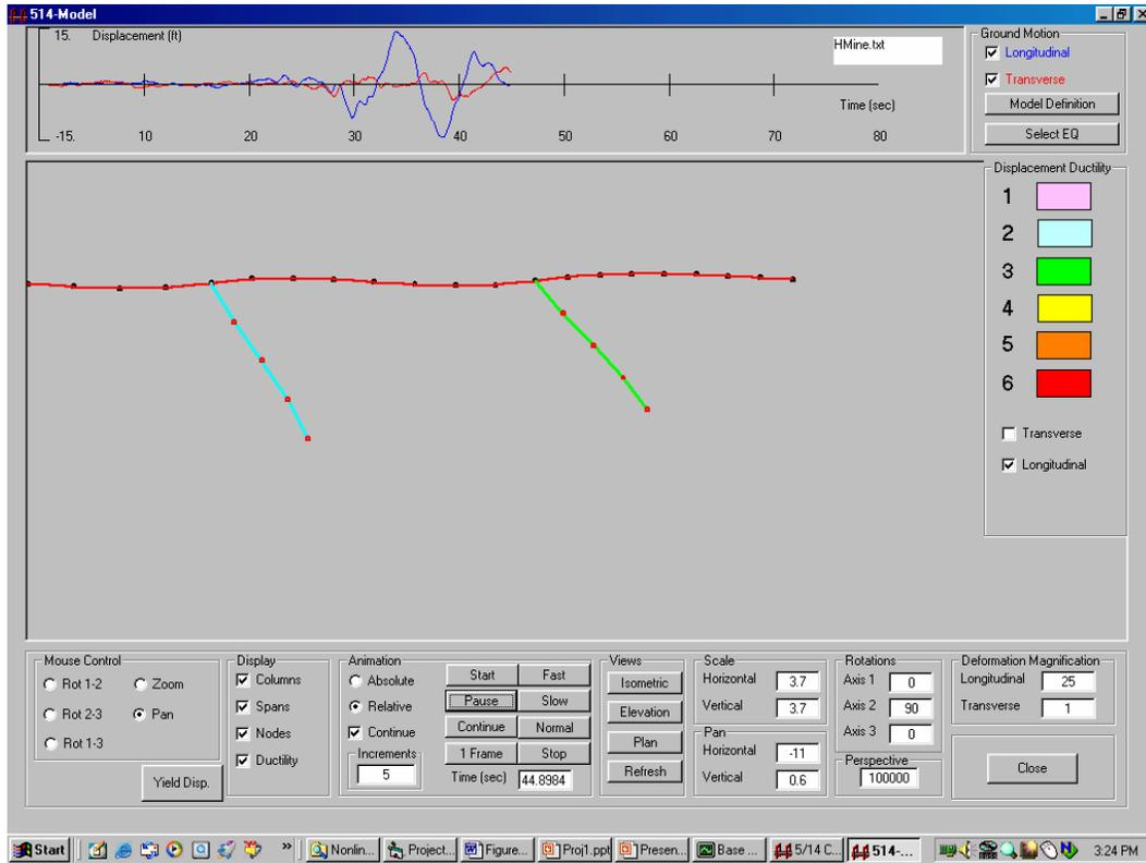
Figure 13. Column at Bent 10 at displacement ductility 3
