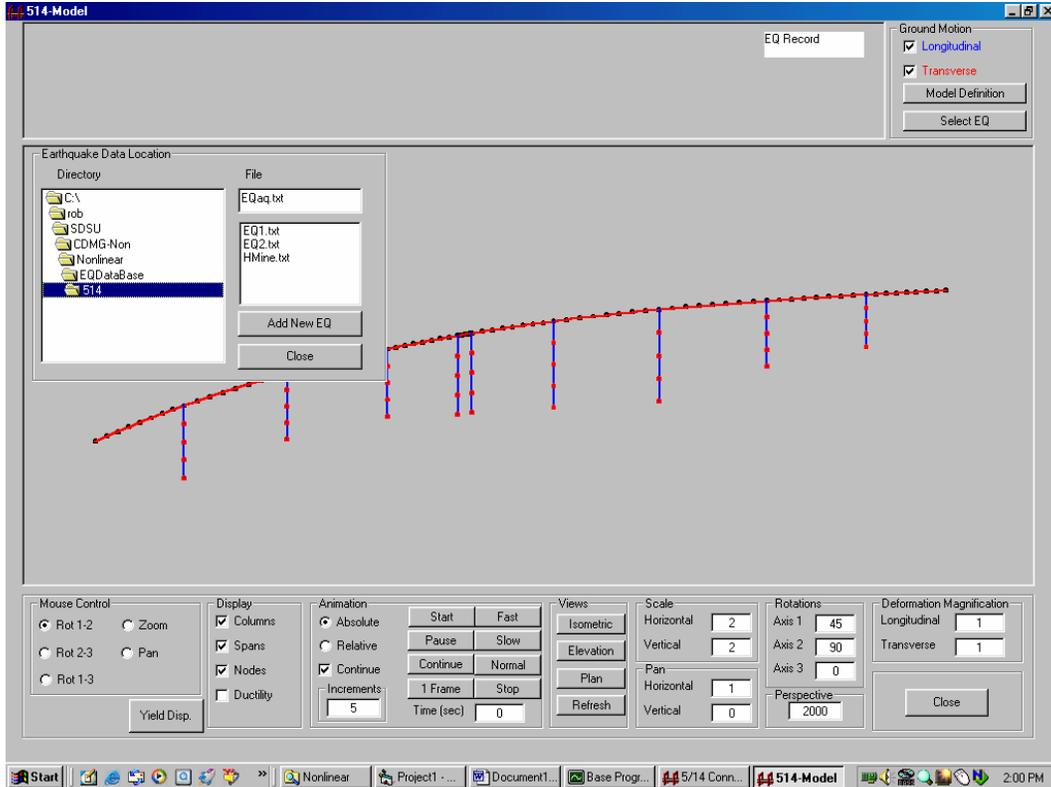
Figure 8. Selection of earthquake file from database directory
