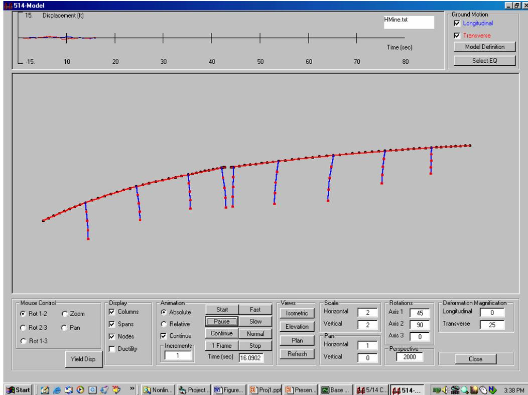
Figure 14. Transverse response prior to plastic column hinging.
