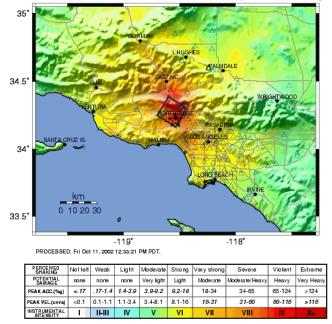
TriNet Rapid Instrumental Intensity Map for Northridge Earthquake Mon Jan 17, 1994 04:30:55 AM PST M 6.7 N34.21 W118.54 Depth: 18.0km ID: Northridge
