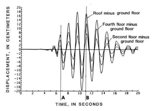
Figure 5. Time history of east-west relative displacement between roof and ground floor (difference of data from accelerometers 4 and 13), between fourth and ground floors (difference of data from accelerometers 5 and 13), and between second and ground floors (difference of data from accelerometers 6 and 13). A and B are interpreted to be the times at which damage initiated and the columns collapsed at the east side of the building (see Figure 3).
