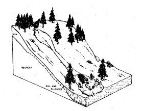
Debris flow: A landslide in which a mass of coarse-grained soil flows downslope as a slurry similar to ready-mixed concrete. Material involved is commonly a loose combination of surficial deposits, rock fragments, and vegetation, including trees. High pore water pressures, typically following intense rain, cause the soil and weathered rock to rapidly lose strength and flow downslope.
