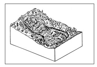
active or historic: The landslide appears to be currently moving or movements have been recorded in the past. Fresh cracks, disrupted vegetation or displaced or damaged man-made features indicate recent activity. Water may be ponded in depressions created by rotation of the slide mass or blockage of stream drainage.
