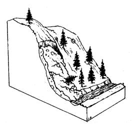
DEBRIS SLIDE: A slide of coarse-grained soil, commonly consisting of a loose combination of surficial deposits, rock fragments, and vegetation. Strength of the material is low, but there may be a very low strength zone at the base of the soil or within the weathered bedrock. Debris slides typically move initially as shallow intact slabs of soil and vegetation, but break up after a short distance into rock and soil falls and flows.
