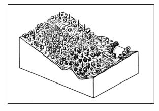
dormant-old: The landforms related to the landslide have been greatly eroded, including significant gullies or canyons cut into the landslide mass by small streams. Original headscarp, benches and hummocky topography are now mostly rounded and subtle. Closed depressions or ponds now filled in. Vegetation has recovered and mostly matches the vegetation outside the slide boundaries.
