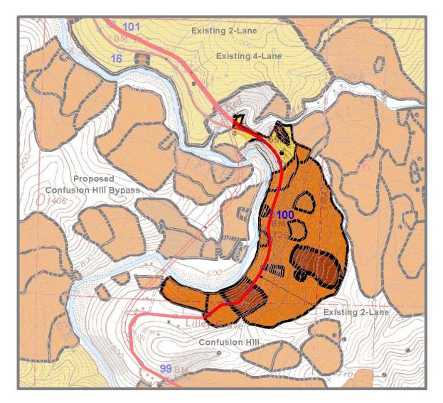
Figure 5b. The existing highway near Confusion Hill is subject to landslides and debris flows, especially at PM 99.8. Recently active slides have resulted in repeated lane closures and traffic control. The proposed bypass would eliminate this segment of Highway 101,
