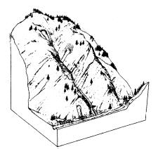
DEBRIS SLIDES and DEBRIS FLOWS are commonly found on a landform called a DEBRIS SLIDE SLOPE, which represents the coalesced scars of numerous landslides that are too small to depict on a map of this scale. These landforms are generally very steep, and have developed in areas of weak bedrock mantled with loose, thin soils and covered with sparse vegetation.
