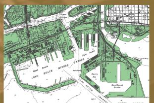
Map of Long Beach area liquefaction hazard zone (green), CGS's Seismic Hazard Program.
