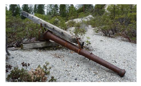
Hydraulic mining was possible after a network of water diversions and ditches was constructed. Then, miners used huge water cannons called "monitors" to wash whole hillsides down into sluice boxes where the gold was recovered. The sluice boxes were embedded at the lowest level of the hydraulic pit, thus the name "ground sluice."
