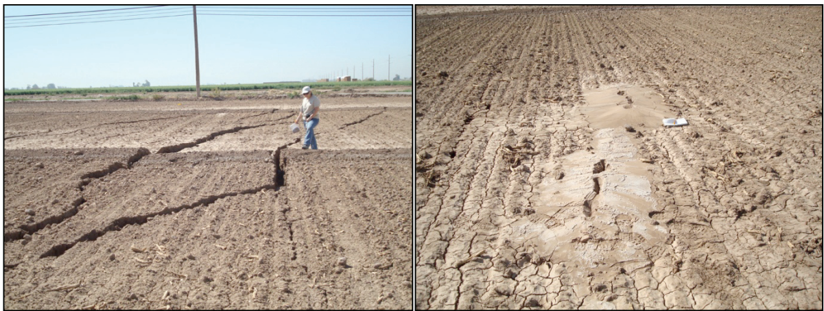
Figure 91. A, Arcuate lateral spread fissures and B, vented sand near the eastern extent of the lateral spread at Rice Drain No. 3 (D12). Photos by T. McCrink, 4/9/10.
