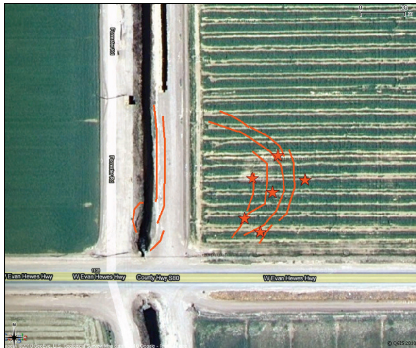
Figure 88. Diagrammatic sketch of liquefaction-related features north of Evan Hewes Highway and east of Rice Drain No. 3 (D12). Lines represent approximate location of cracks and fissures, and star symbols indicate approximate location of sand boils. Base image is from Google Maps; Google label for Forrester Road appears to be in error.
