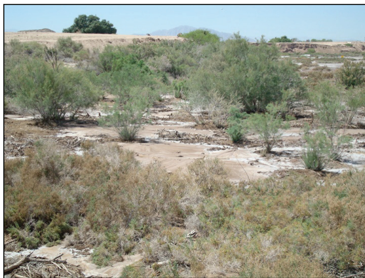
Figure 113. Extensive vented sand flooding areas between bushes on the New River floodplain west of the waste water treatment plant (F04). View to the west. Photo by T. McCrink, 4/10/10.
