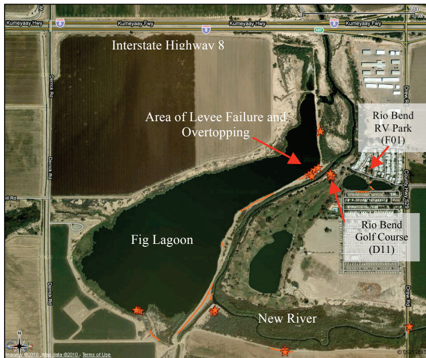
Figure 80. Diagrammatic sketch of liquefaction-related features in the vicinity of Fig Lagoon (D10). Red lines represent lateral spread cracks and red stars represent areas of vented sand. Fig Lagoon lies south of Interstate Highway 8, west of Drew Road, and east of Derrick Road. Also shown are the Rio Bend RV Park and Rio Bend Golf Course sites, which will be discussed in under site entries F01 and D11 respectively. Base image is from Google Maps.
