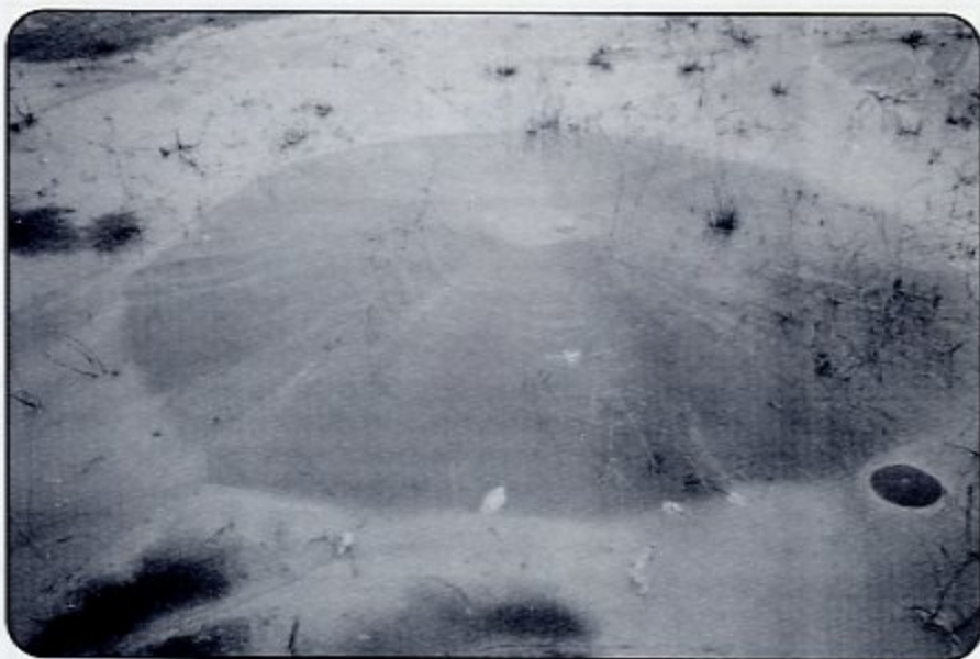
Photo 3. "Flowing" sand boil. At about noon on April 18, 1990 several sand boils were still active. When this photo was taken, water was still issuing from the central crater of this sand boil and flowing evenly over all sides of the volcano-shaped mound (note ripples on the sides of the sand boil).
