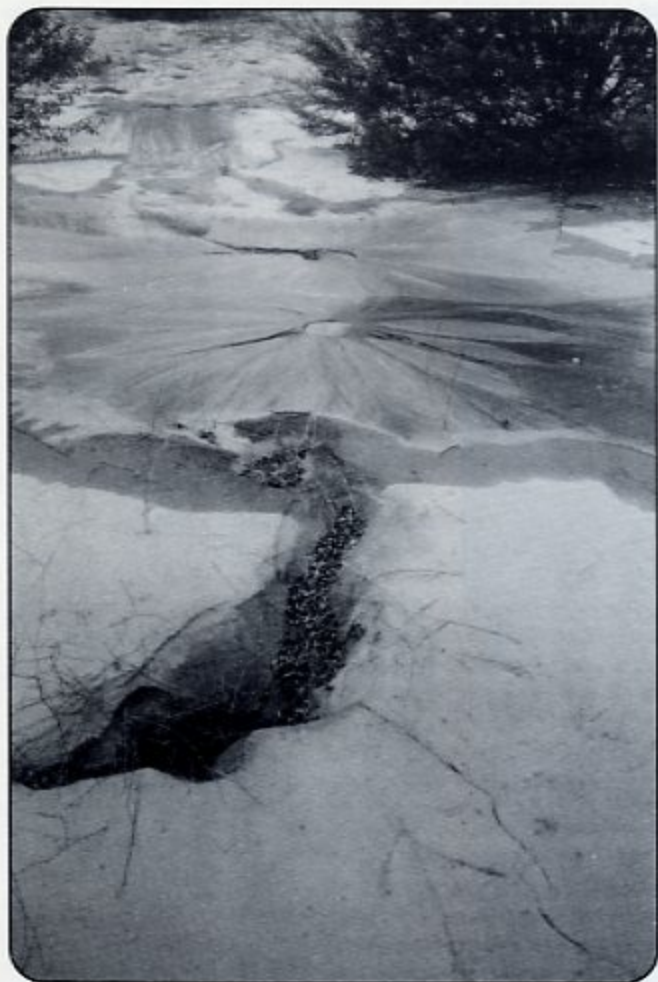
Photo 4. Sand boil formed by the Loma Prieta earthquake (central fissure in foreground) with two sand boils that were erupted on April 18, 1990, possibly from the same fissure.
