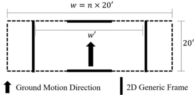
Figure 3. Modeling approach to capture plan aspect ratio
