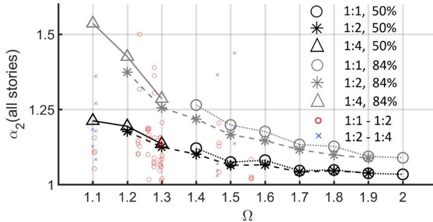
Figure 8. Analytical and CSMIP data of  $\alpha_{2,all}^{50\%}$  and  $\alpha_{2,all}^{84\%}$  with respect to  $\Omega$  and plan aspect ratio for 4-story buildings subject to ground motions of 72-year average return period
