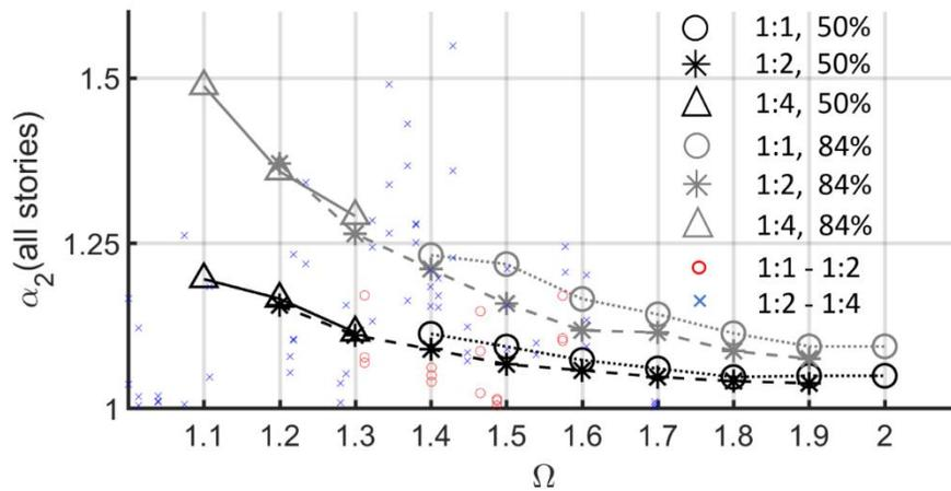
Figure 7. Analytical and CSMIP data of  $\alpha_{2,all}^{50\%}$  and  $\alpha_{2,all}^{84\%}$  with respect to  $\Omega$  and plan aspect ratio for 4-story buildings subject to ground motions of 72-year average return period
