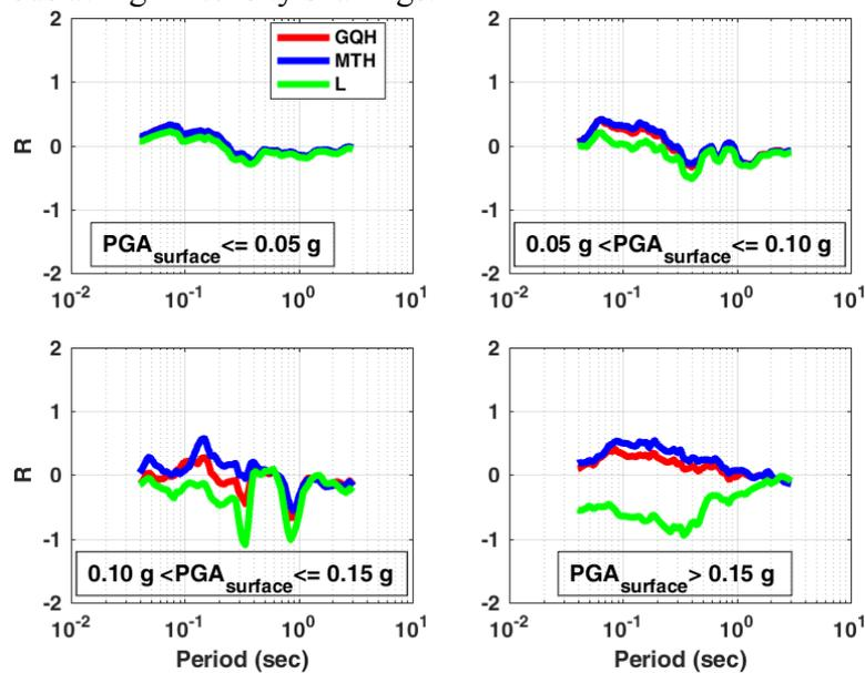
Figure 11. Computed mean residual of amplification factor for all sites at different ranges of measured  $PGA_{\text{surface}}$ .
