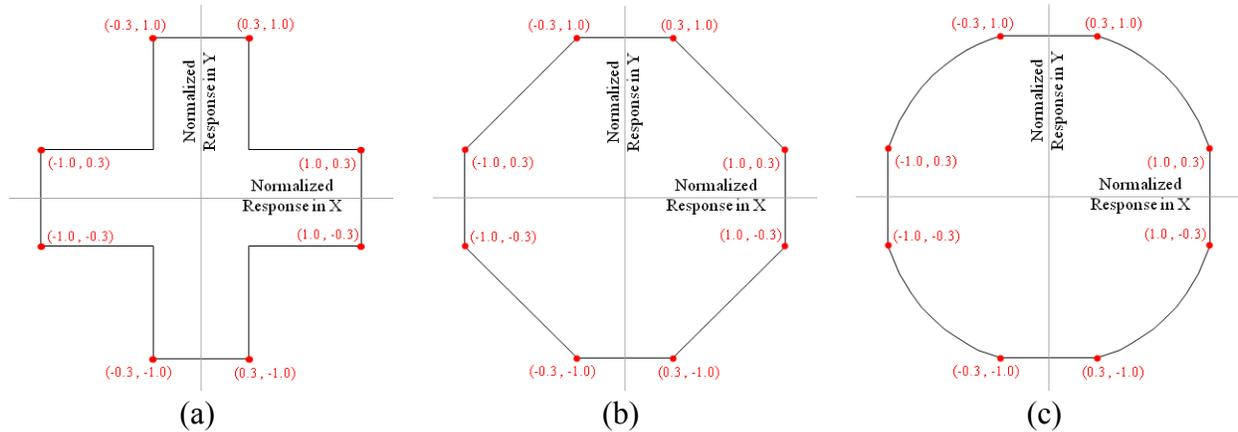
**Figure 3.** Interpolation of the eight control points in the ASCE/SEI 7-10 direction of loading provisions based on (a) no interpolation on the diagonal, (b) linear interpolation on the diagonal and (c) elliptical interpolation on the diagonal. Control points shown as red dots.
