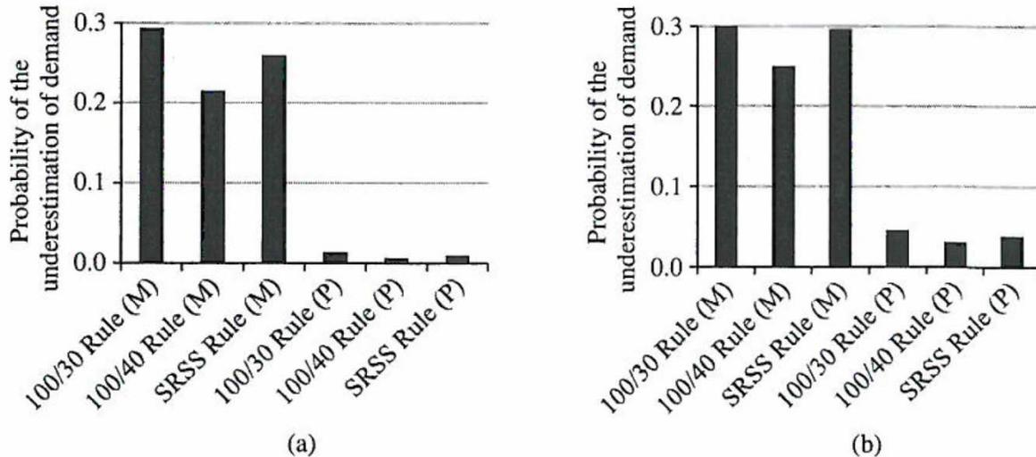
**Figure 2.** Probability of underestimation of (a) displacement and (b) force demands for SRSS, 100%+30% and 100%+40% combination rules. Letter M denotes only the major component of earthquake was used (Case 1) and letter P denotes that the paired record was used (Case 2). This figure is a direct reproduction of Figure 8 in Bisadi and Head (2011).
