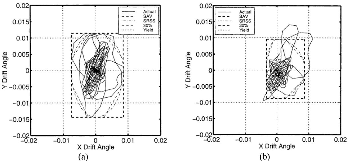
**Figure 1.** Results and combination rules for (a) linear and (b) nonlinear response history analysis. Note that (a) and (b) use a different angle of ground motion application to the building which explains why the combination rule envelopes differ. This figure is direct reproductions of Figure 4 and Figure 5, respectively, in MacRae and Tagawa (2001).
