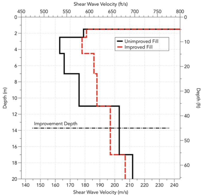
Figure 9b: Comparison of shear wave velocity profiles focusing on zones of unimproved hydraulic fill and adjacent fill improved with stone columns.
