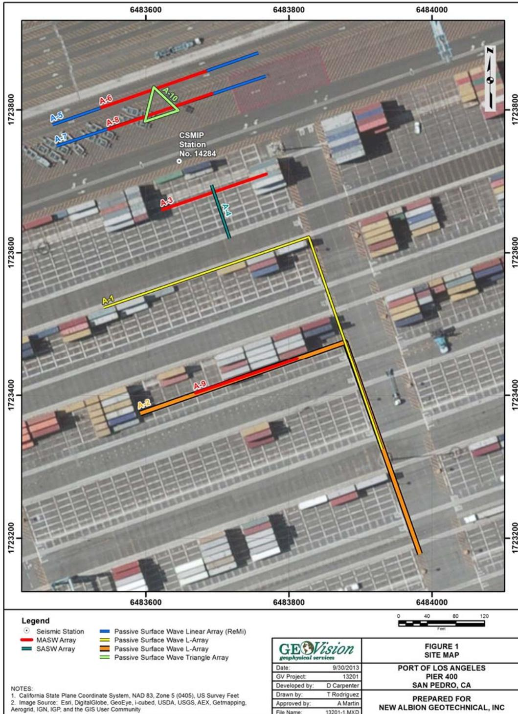
Figure 7: Location of geophysical arrays for surface wave velocity investigation at Port of Los Angeles Berth 404 (GEOVision 2013).
