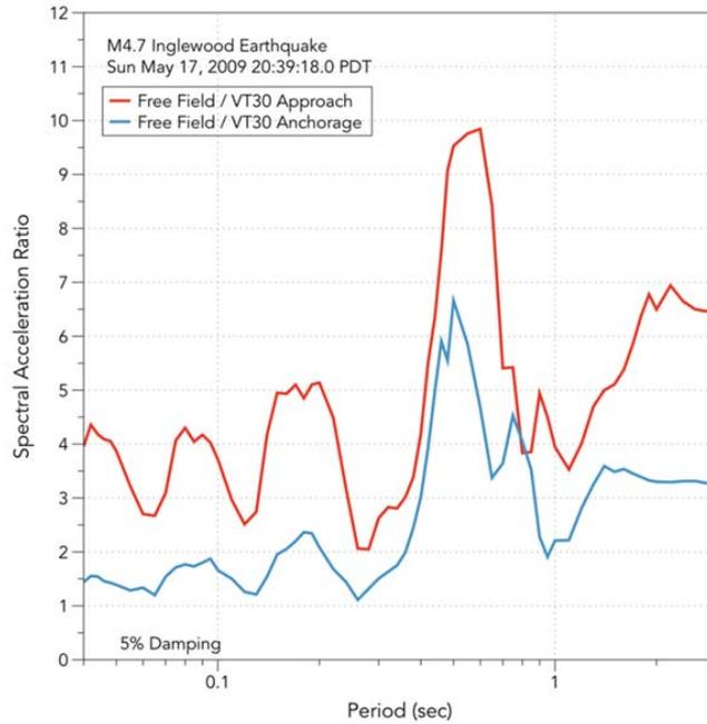
Figure 6a: Spectral amplification ratios for free-field ground surface motion at Berth 404 and motions recorded at a depth of 100 ft at the Vincent Thomas Bridge West Arrays.
