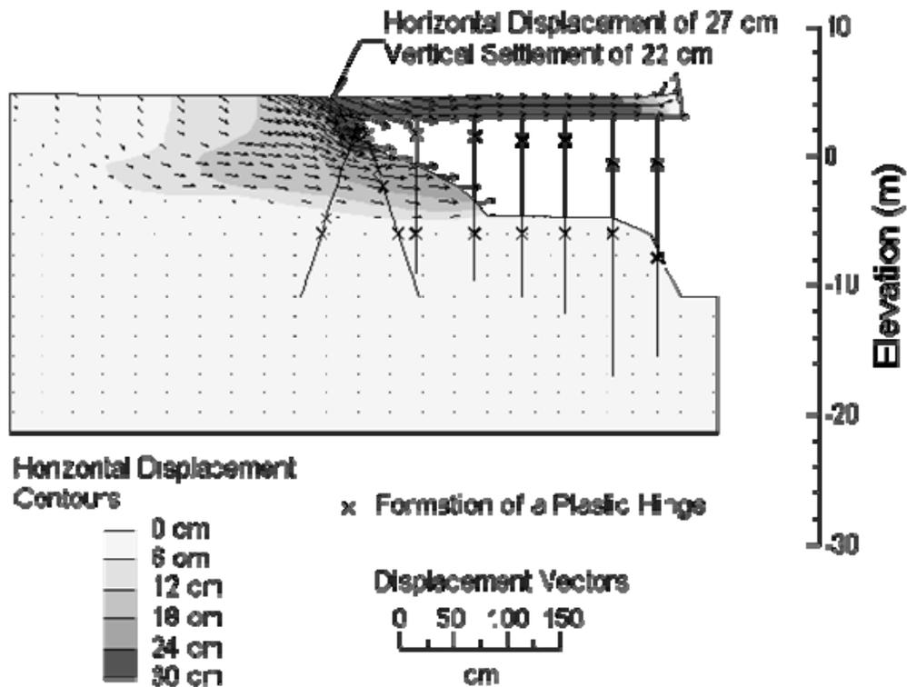
Figure 3. Numerical simulation of seismic performance of Berth 38, Seventh Street Terminal, Port of Oakland during the 1989 Loma Prieta Earthquake.
