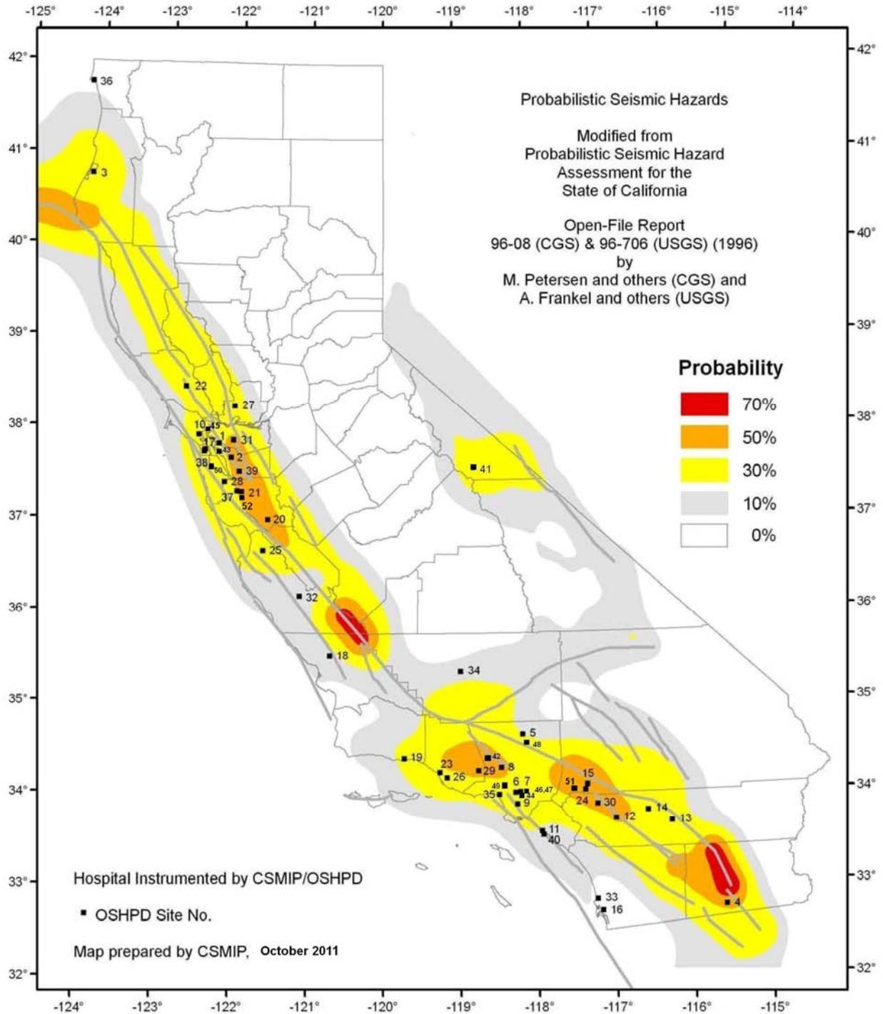
Figure 3. Instrumented Hospital Buildings by SMIP/OSHPD for sites with PGA > 0.2g in 20 years on alluvial soil conditions.
