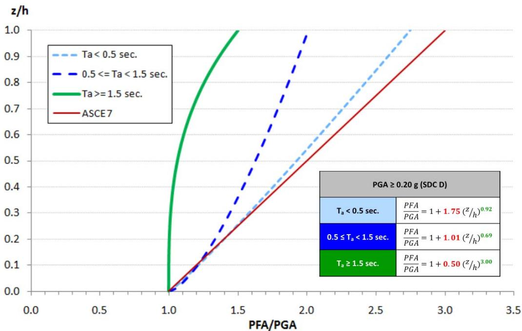
**Figure 7. Profile of PFA/PGA over Building Height Recommended for Seismic Design of Acceleration-Sensitive Nonstructural Components in New Constructions under Earthquakes with PGA ≥ 0.20 g (SDC D or Higher of Occupancy Category I through III)**
