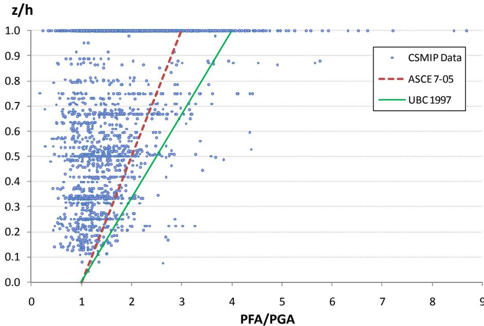
**Figure 2. Data Points vs. Building Code Formula for Relationship between PFA/PGA and  $z/h$  (2224 above-Ground Level Data Points from 151 Fixed-Base Building Stations)**
