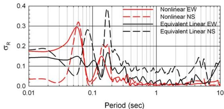
**Figure 7. Estimated model-to-model uncertainty for equivalent linear and nonlinear predictions of ground surface motions.**
