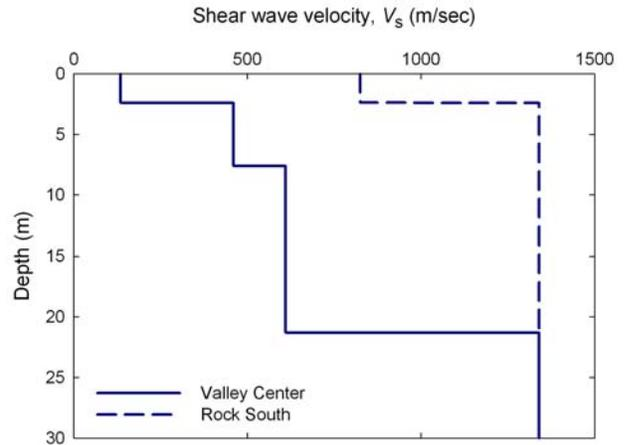
Figure 2. Standard shear wave velocity profiles for Valley Center and Rock South locations (after Real, 1988).
