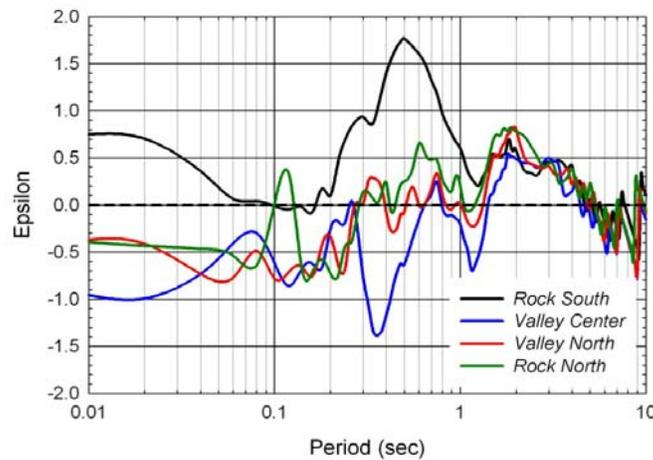
Figure 9. Epsilon values for four Turkey Flat rock outcrop motions. Median spectral accelerations calculated using Campbell and Bozorgnia (2009) with  $V_{s,30} = 1,276$  m/sec,  $Z_{2.5} = 0.27$  km,  $M_w = 6.0$ , and  $R = 7.6, 8.2, 8.6,$  and  $9.2$  km.
