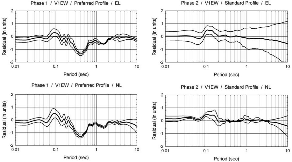
**Figure 6. Residuals for Phase 1 and 2 equivalent linear and nonlinear analyses of V1 ground motions using preferred soil models. Bold line indicates mean and lighter lines indicate mean  $\pm \sigma_{\ln R}$ .**
