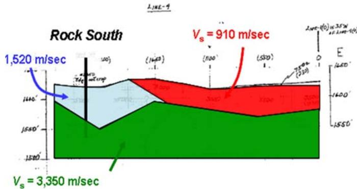
Figure 10. Inferred velocity profile in vicinity of Rock South recording instrument (after Real, 1988).
