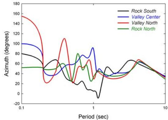
Figure 11. Azimuthal orientation of maximum spectral acceleration. Azimuthal angle is measured clockwise from north-south direction.
