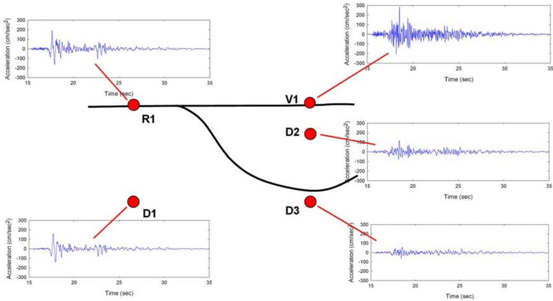
**Figure 3. Time histories of North-South accelerations recorded at Rock South and Valley Center downhole arrays in September 28, 2004 Parkfield earthquake.**
