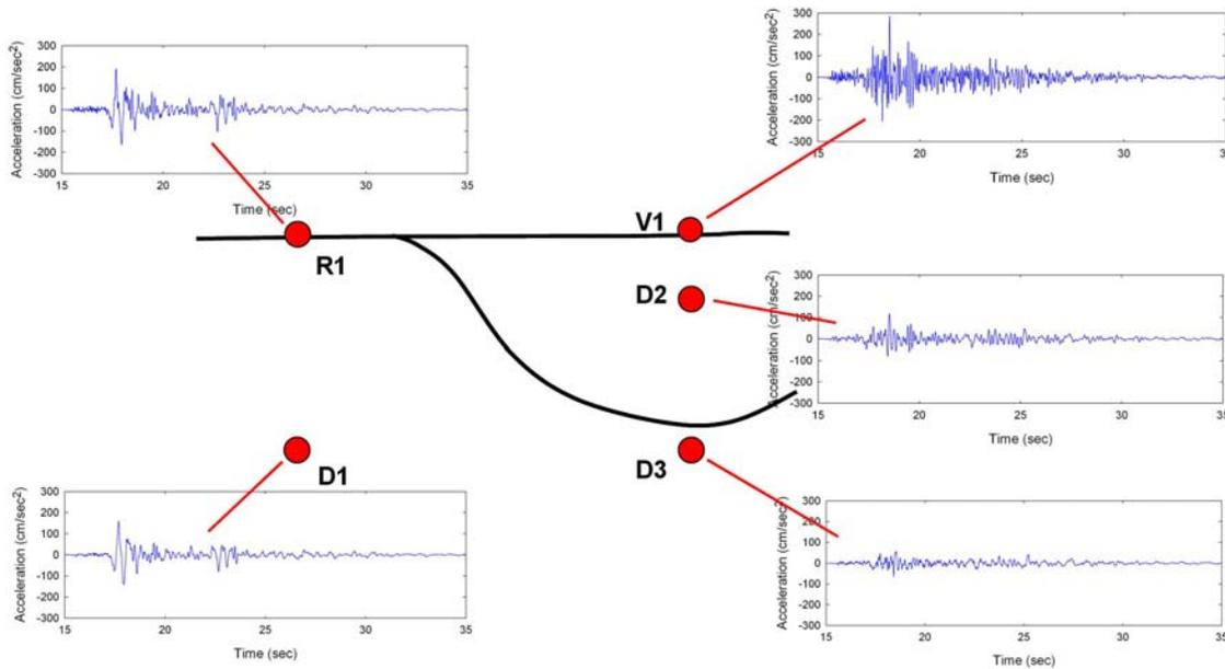
**Figure 4. Time histories of North-South accelerations recorded at Rock South and Valley Center downhole arrays in September 28, 2004 Parkfield earthquake.**
