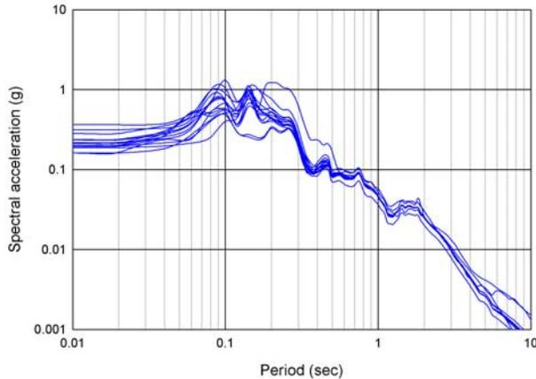
**Figure 8. Equivalent linear predicted NS motions at surface of Valley Center site. Mean predicted spectrum indicated by bold line.**
