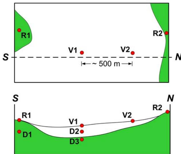
Figure 1. Schematic illustration of Turkey Flat instrumentation layout (after Tucker and Real, 1986).
