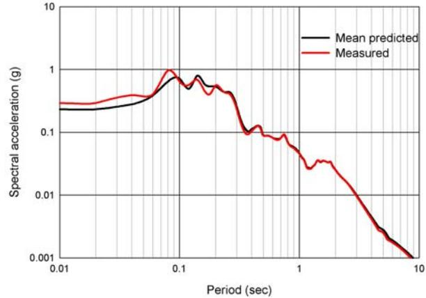
**Figure 9. Recorded and mean equivalent linear predicted NS motions at surface of Valley Center site.**
