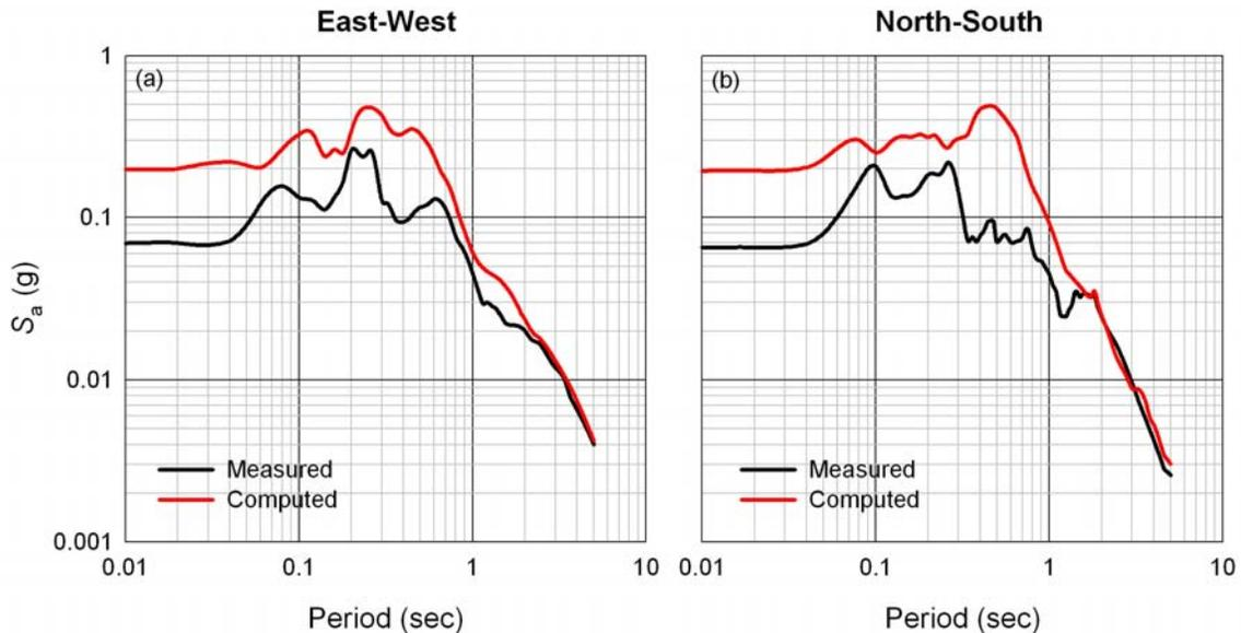
**Figure 12.** Measured and computed response spectra at location of D3 instrument. Computed motions are within-profile measurements based on measured R1 motions.
