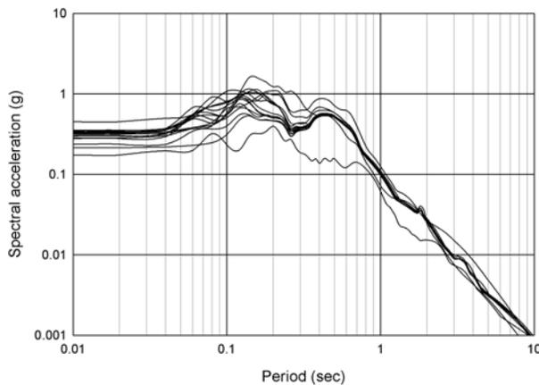
**Figure 6. Equivalent linear predicted NS motions at surface of Valley Center site. Mean predicted spectrum indicated by bold line.**
