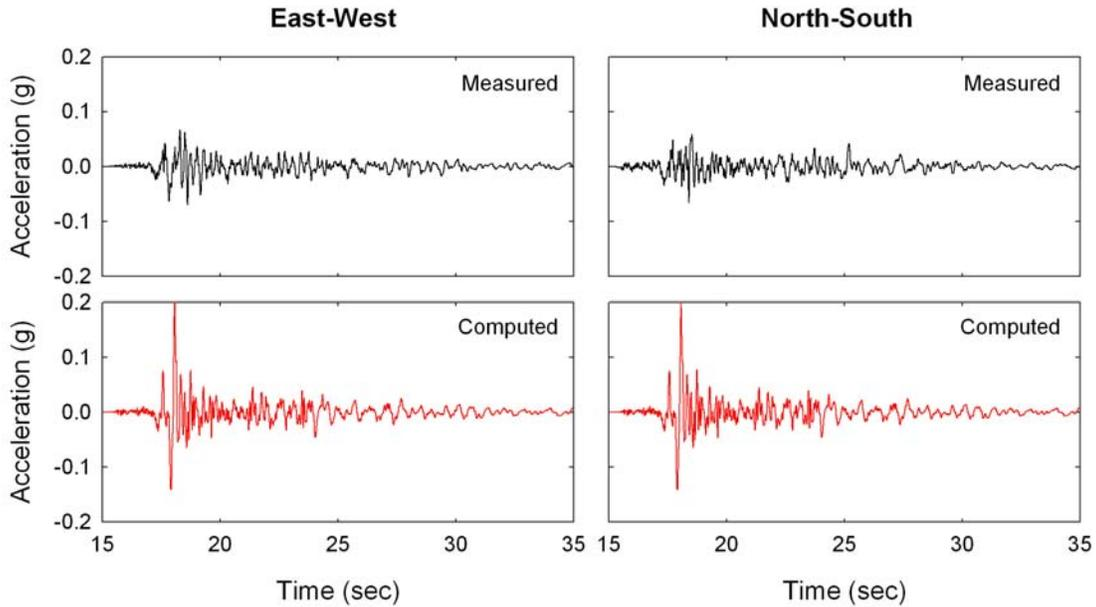
**Figure 11.** Measured and computed motions at location of D3 instrument. Computed motions are within-profile measurements based on measured R1 motions.
