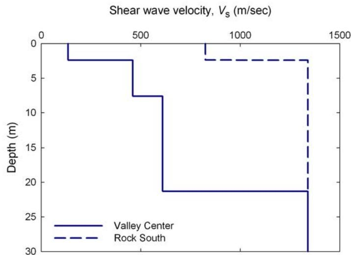
**Figure 3. Standard shear wave velocity profiles for Valley Center and Rock South locations (after Real, 1988).**
