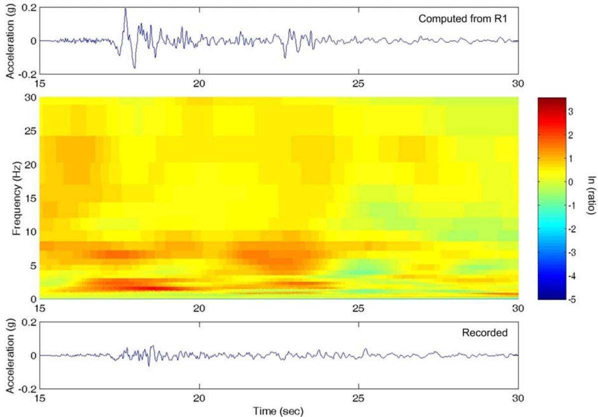
**Figure 13. Time histories of NS component of D3 motion computed from R1 motion and recorded, and ratio of wavelet amplitudes (computed:recorded).**
