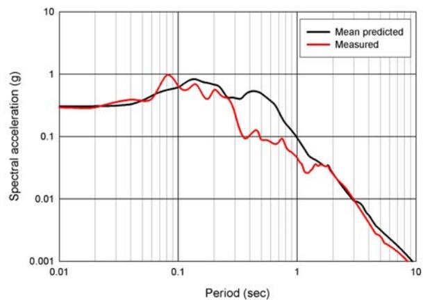
**Figure 7. Recorded and mean equivalent linear predicted NS motions at surface of Valley Center site.**
