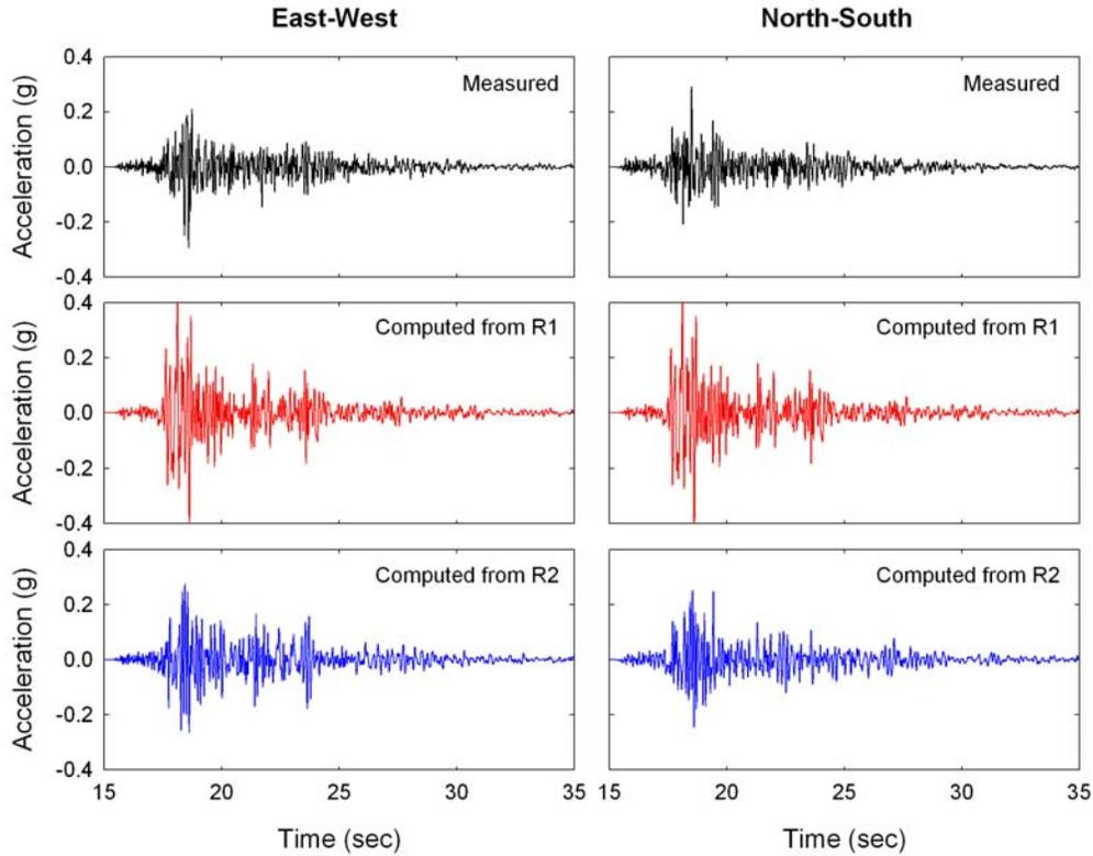
Figure 14. Measured and computed time histories for V1 instrument at Valley Center site.
