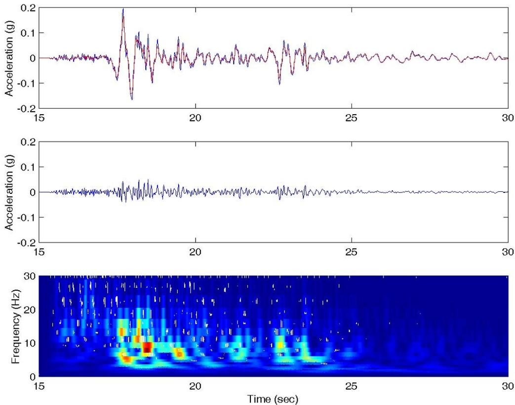
**Figure 10. Rock South profile measurements: (upper) R1 (blue) and D1 (red) motions; (middle) R1 – D1 motion; and (lower) wavelet amplitudes vs. frequency and time for R1 – D1 motion.**
