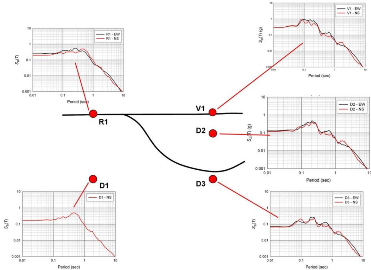
**Figure 5. Response spectra from motions recorded at Rock South and Valley Center downhole arrays in September 28, 2004 Parkfield earthquake. EW component of D1 instrument was not recorded due to instrument malfunction.**
