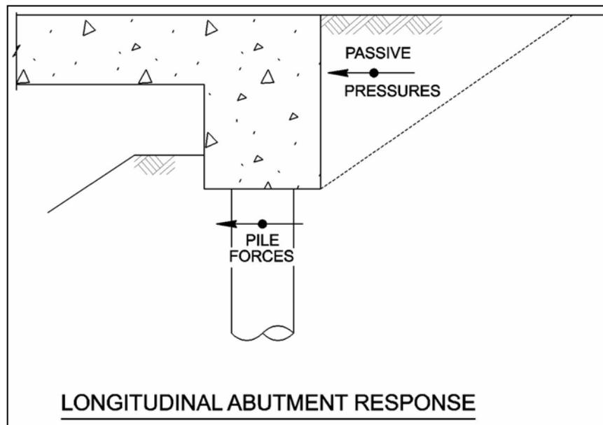
Figure 8. Longitudinal Forces at Abutment
