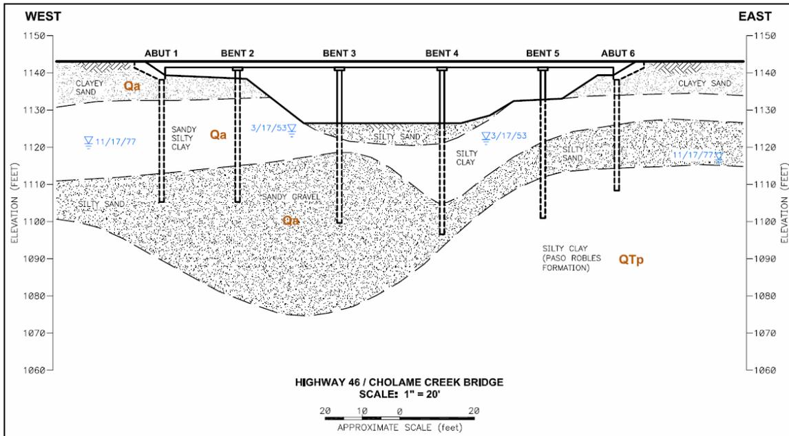
Figure 2. Bridge Elevation and Subgrade Conditions
