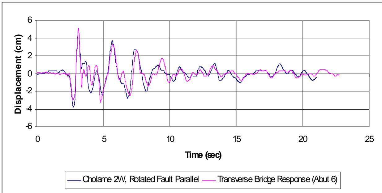
Figure 11. Measured Displacement Time History Comparison in Transverse Direction
