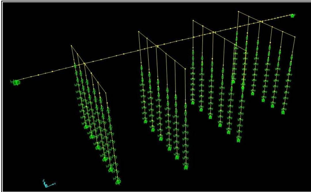
Figure 7. SAP2000 Model of Bridge Structure with Soil-Pile Springs
