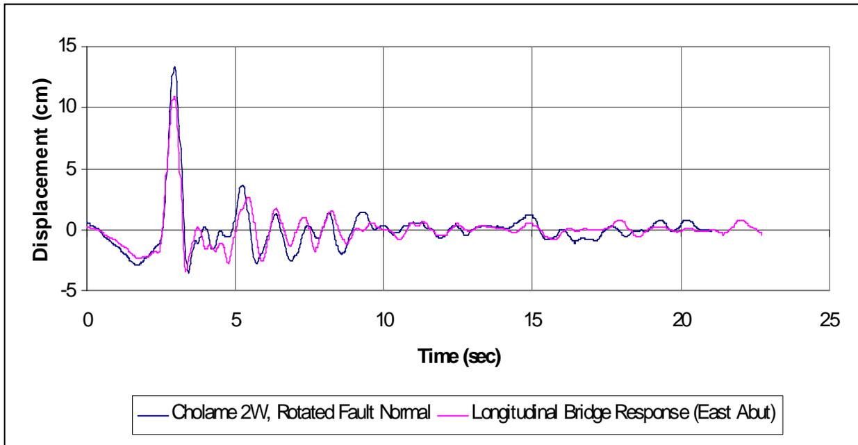
Figure 10. Measured Displacement Time History Comparison in Longitudinal Direction
