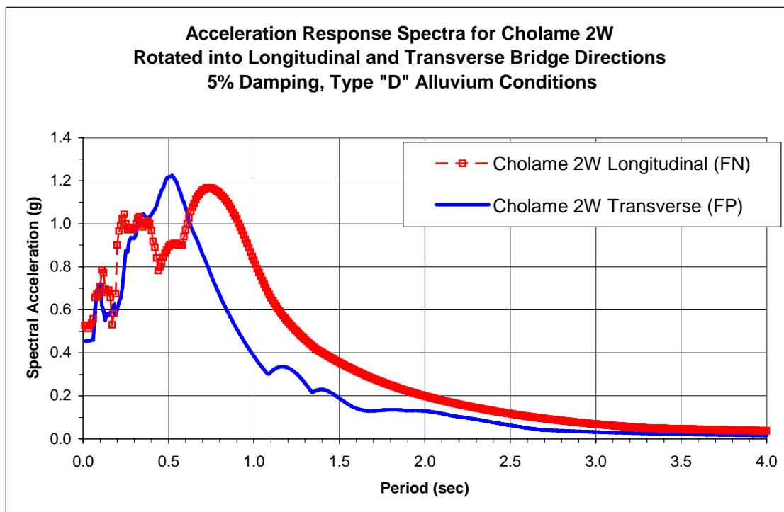
**Figure 6. Cholame 2W Acceleration Response Spectra for 2004  $M_w$  6.0 Event**
