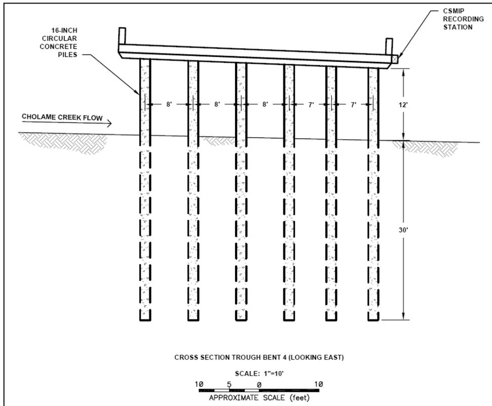
Figure 3. Bridge Cross Section
