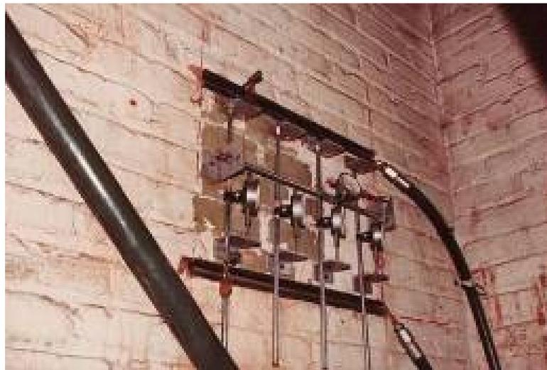
**Figure 6: URM in-stu test setup**
