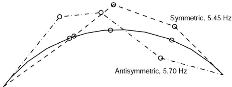
**Figure 8. Symmetric and antisymmetric mode shapes determined from forced vibration testing, the open circles are the locations of the crest level stations**
