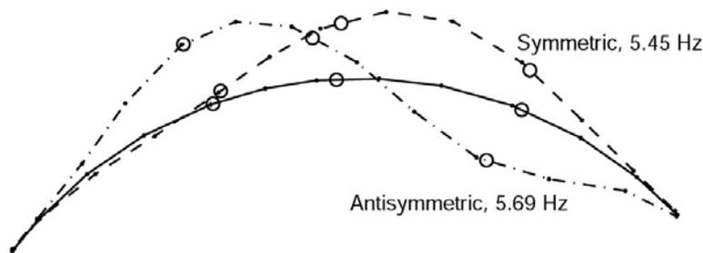
**Figure 10. Symmetric and antisymmetric mode shapes computed from linear SCADA model calibrated to match forced vibration modal parameters, the open circles are the locations of the crest level stations**
