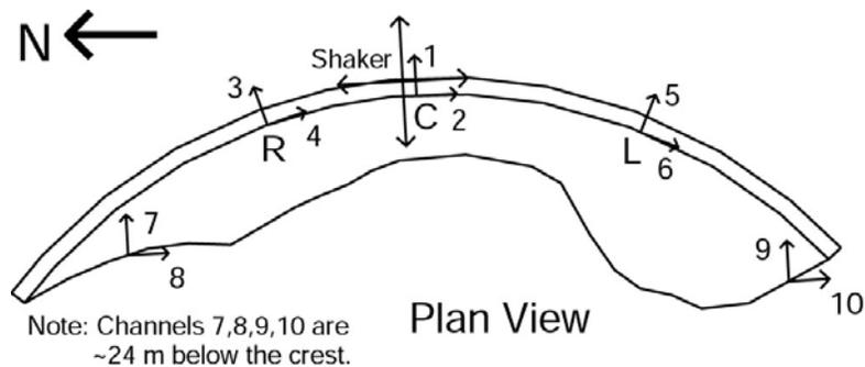
**Figure 6. Ranger and shaker force locations and directions**
