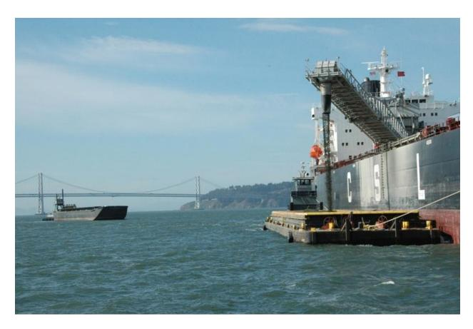
Freighter delivering 79,200 tons of high-grade construction aggregate from Polaris Minerals' Orca Quarry on Vancouver Island, British Columbia to the San Francisco Bay area market. Aggregate is off loaded to barges at a rate of 4,500 tons per hour. The cost of shipping a ton of aggregate 1,000 miles by freighter is about equivalent to the cost to transporting it 25 miles by truck in the Bay area. **Photo courtesy of Polaris Minerals.**
