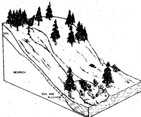
**Debris flow:** A landslide in which a mass of coarse-grained soil flows downslope as a slurry similar to ready-mixed concrete. Material involved is commonly a loose combination of surficial deposits, rock fragments, and vegetation, including trees. High pore water pressures, typically following intense rain, cause the soil and weathered rock to rapidly lose strength and flow downslope.
