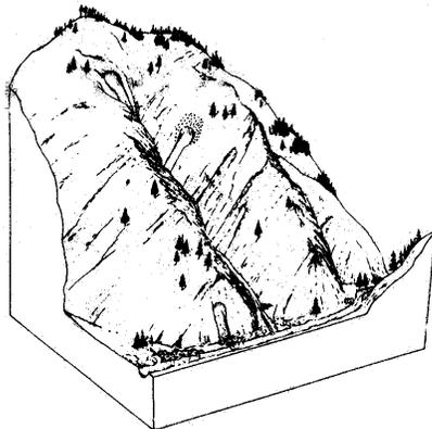
DEBRIS SLIDES and DEBRIS FLOWS are commonly found on a landform called a DEBRIS SLIDE SLOPE, which represents the coalesced scars of numerous landslides that are too small to depict on a map of this scale. These landforms are generally very steep, and have developed in areas of weak bedrock mantled with loose, thin soils and covered with sparse vegetation.
