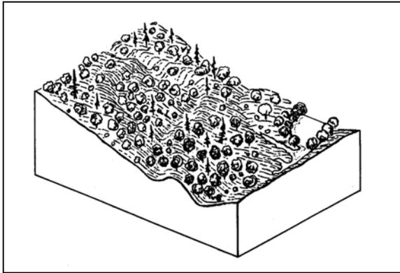
dormant-old: The landforms related to the landslide have been greatly eroded, including significant gullies or canyons cut into the landslide mass by small streams. Original headscarp, benches and hummocky topography are now mostly rounded and subtle. Closed depressions or ponds now filled in. Vegetation has recovered and mostly matches the vegetation outside the slide boundaries.
