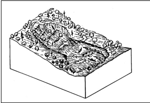
active or historic: The landslide appears to be currently moving or movements have been recorded in the past. Fresh cracks, disrupted vegetation or displaced or damaged man-made features indicate recent activity. Water may be ponded in depressions created by rotation of the slide mass or blockage of stream drainage.
