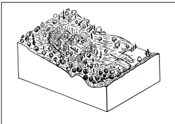
dormant-mature: The landforms related to the landslide have been smoothed by erosion and re-vegetated. The main scarp is rounded, the toe area has been eroded and some new drainages established within the slide area. Benches and hummocky topography on the slopes are subdued and commonly obscured by dense, relatively uniform vegetation.
