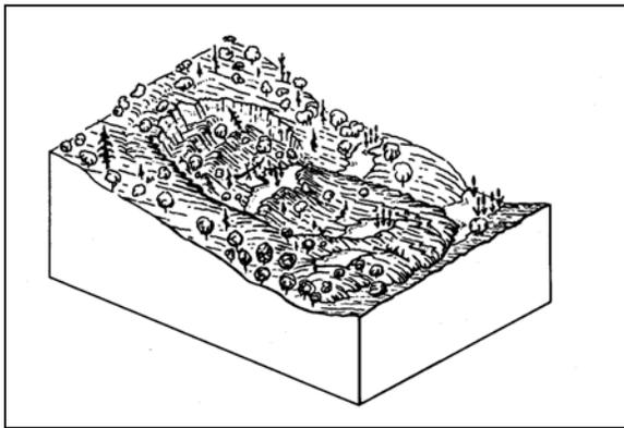
dormant-young: The landforms related to the landslide are relatively fresh, but there is no record of historic movement. Cracks in the slide mass are generally absent or greatly eroded; scarps may be prominent but are slightly rounded. Depressions or ponds may be partly filled in with sediment, but still show phreatophytic vegetation.
