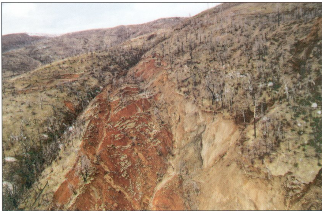
Photo 3. Axial view N20°W of the upper half of Mill Creek landslide showing debris slide blocks and translational movement. Note structural control of west side of landslide (at left) and asymmetric tilt of slide mass. Prominent joint-controlled bedrock gully at left. Reddish-brown colluvium (derived from pyroxenite) within the debris slide contrasts in color with gray colluvium derived from diorite and schist at right side. Photo by Robert H. Sydnor.
