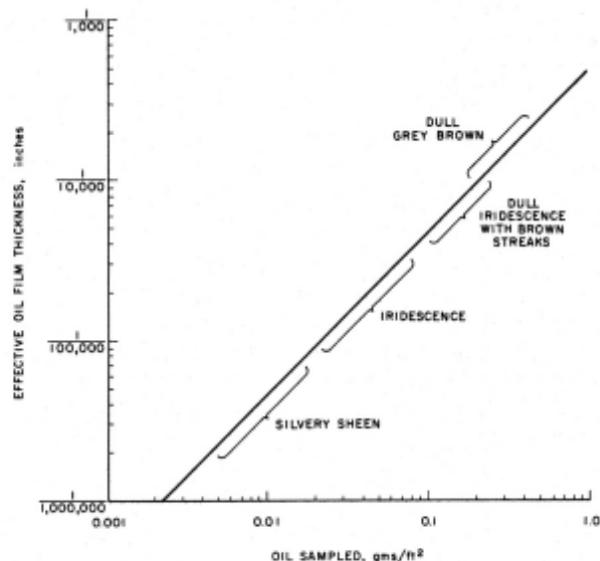
Figure 8. — Oil film appearance and effective thickness as a function of the mass of oil collected ( $\rho = 0.9 \text{ gm/cc}$ ) taken from technical memorandum 1230, General Research Corporation.
