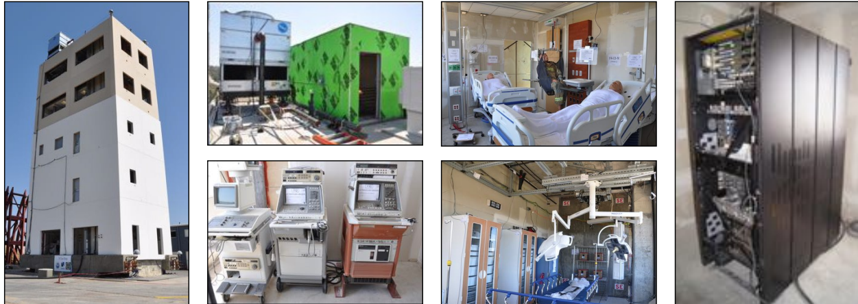
Figure 7. Shake table tests of a five-story reinforced concrete building outfitted with a variety of nonstructural components: test building (left), cooling tower and penthouse of the roof level (top middle left), medical ultrasound imagers of level 4 (bottom middle left), medical equipment of level 4 (top middle right), medical equipment of level 5 (bottom middle right), and computer server at level 3 (right).
