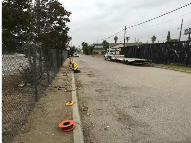
Figure 18 – View of laying out MASW.
