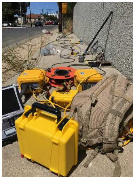
Figure 4 – View of equipment for MASW survey.
