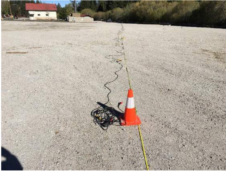
Figure 24 – View of 2D Passive layout.
