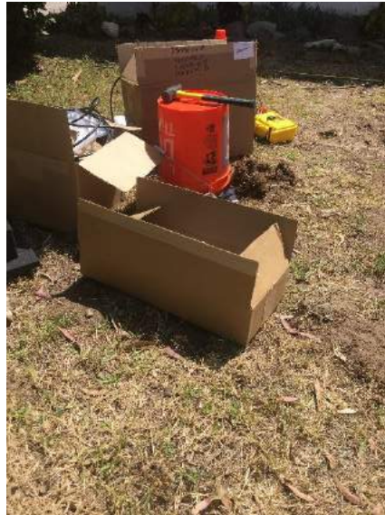
Figure 8 – View of HVSR setup, in ground, thermal protection, and weighted bucket for wind protection.
