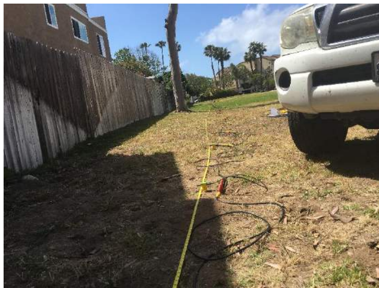
Figure 9 – View of MASW – 5 foot (1.524 meters) spacing on geophones
