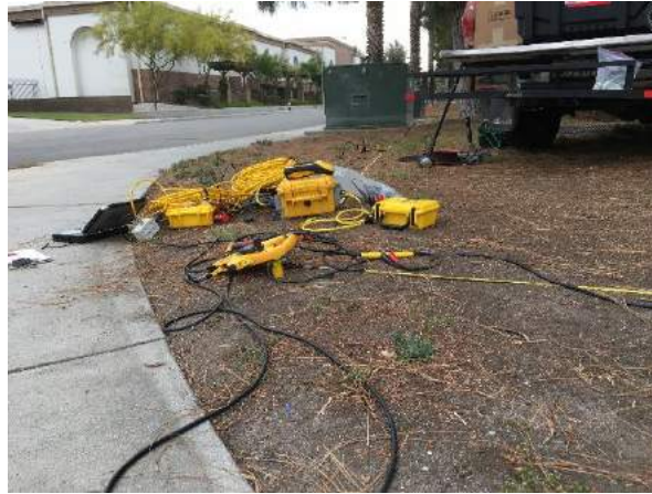
Figure 16 – View of seismic equipment and setup for 2D Passive.
