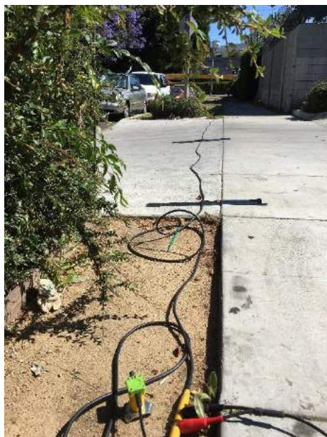
Figure 5 – View of geophones and alignment of 2D Passive line.
