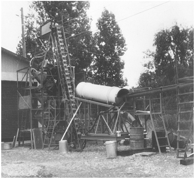
Photo 8. Test plant consisting of a PMX helix (center) and 4 vertically stacked PMX rotary tables (in framework at left). Plant has since been disassembled.
