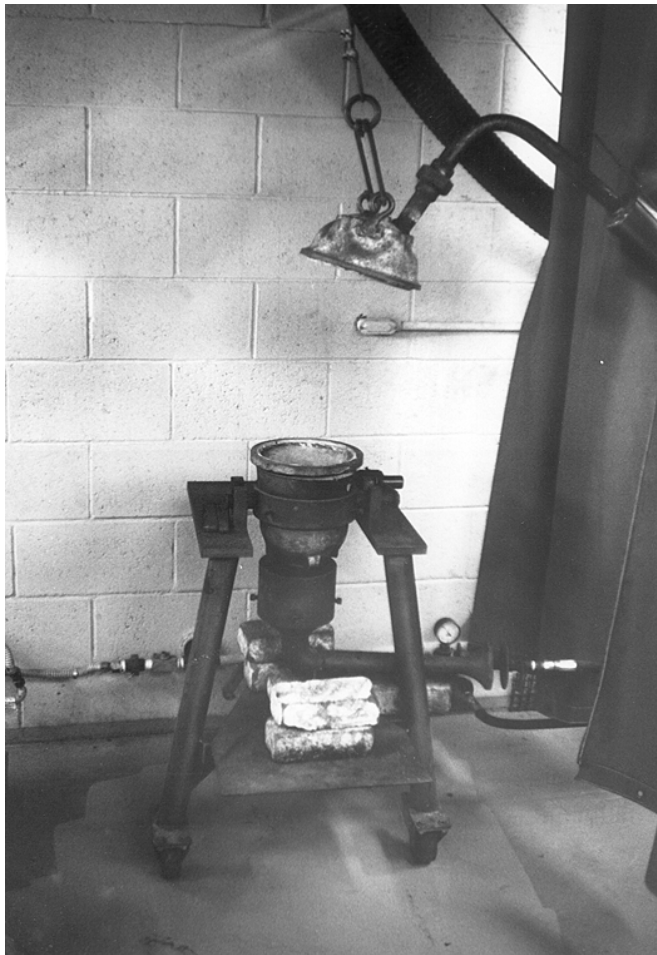
Photo 14. This retort is used to separate gold from the amalgam collected on the dredge.
