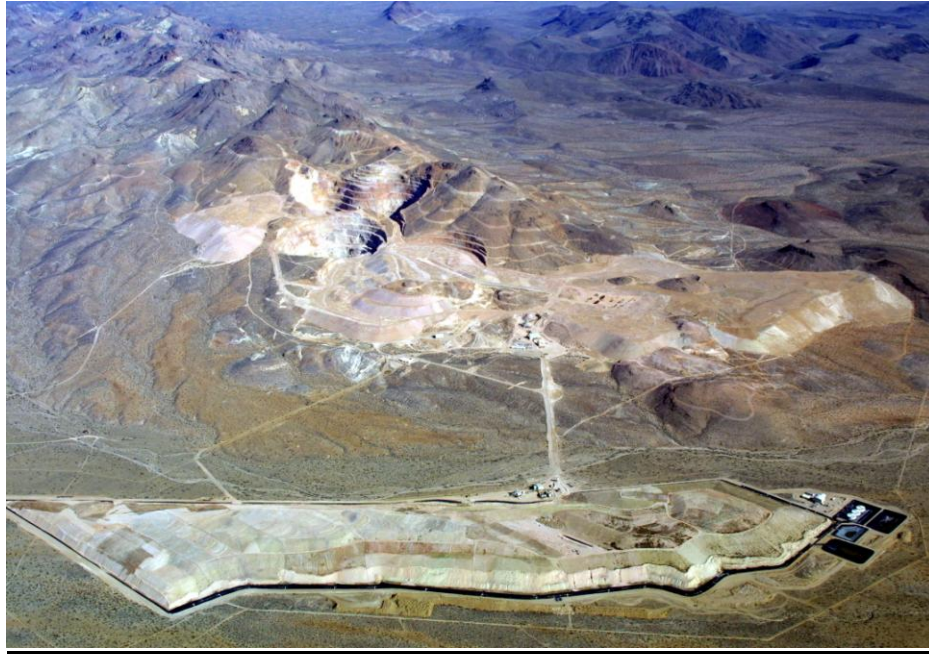
Figure 5a. Castle Mountain Mine was comprised of three open pits, one of which was backfilled. The cyanide leach pad in the foreground is approximately 7700 by 1675 feet in dimension (about 265 acres), and attains a height of 180 feet.
