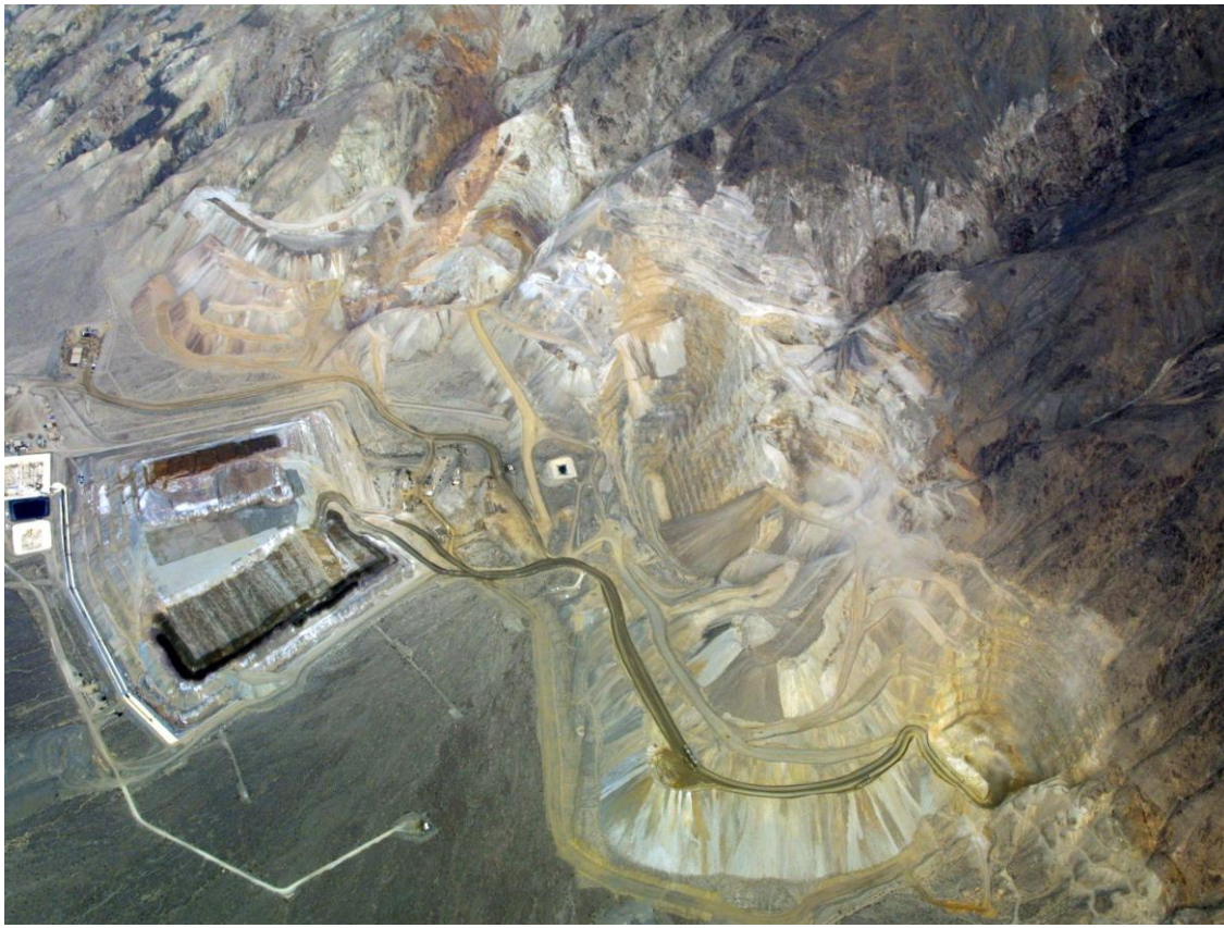
Figure 6. Canyon Resources Briggs Mine is located in the Panamint Range of Southern California. The pit encompasses about 140 acres, and the cyanide leach pads encompass about 137 acres.
