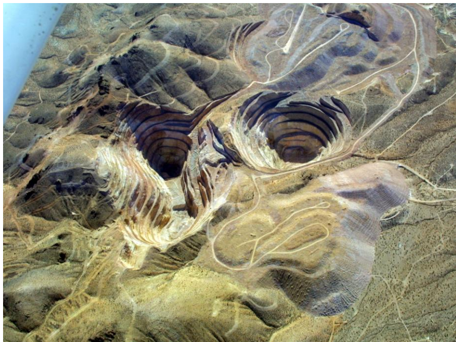
Figure 5a. Castle Mountain Mine was comprised of three open pits, one of which was backfilled. The cyanide leach pad in the foreground is approximately 7700 by 1675 feet in dimension (about 265 acres), and attains a height of 180 feet.
