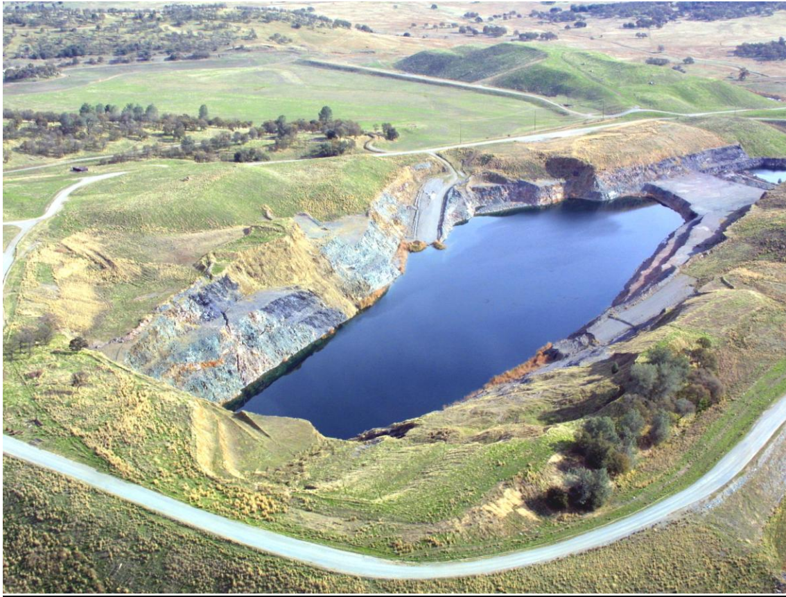
Figure 3. The reclaimed Royal Mountain King Mine is located near Copperopolis, California. The pit is approximately 1600 by 500 feet in dimension, and 400 feet in depth. High arsenic levels are reported for the pit water.
