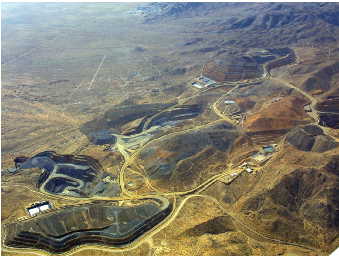
Figure 7a. The Rand Mine located near Randsburg, California. Two open pits are evident, along with a cyanide leach pad in the lower right, and two large waste piles in the central portion of the image. The larger cyanide leach pad in the upper right of the image is about 1.8 by 2.1 miles in extent.
