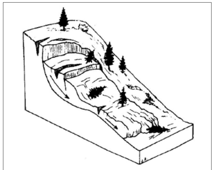
Figure 1. Diagrammatic sketch of a translational/rotational landslide. Drawing by Janet Appleby Richard Killbourne and Thomas Spittler; modified from Varnes (1978)
